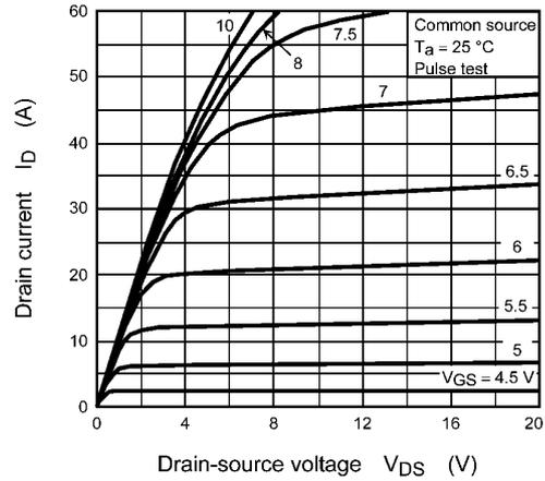
**Fig. 8.2  $I_D - V_{DS}$**
