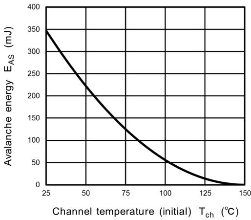
Fig. 8.14  $E_{AS} - T_{ch}$
