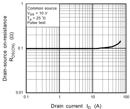
**Fig. 8.6  $R_{DS(ON)} - I_D$**
