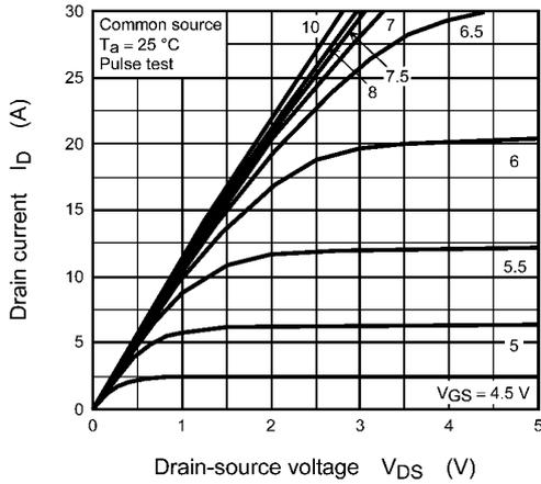
**Fig. 8.1  $I_D - V_{DS}$**
