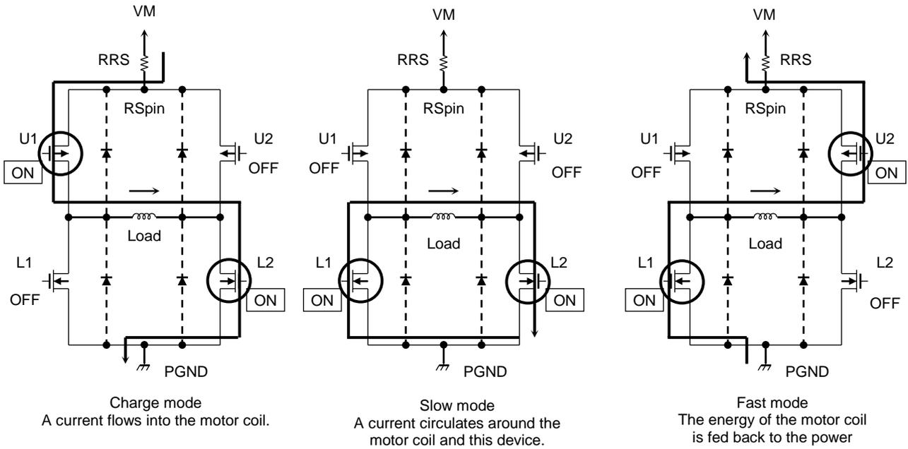
**Output transistor function**
