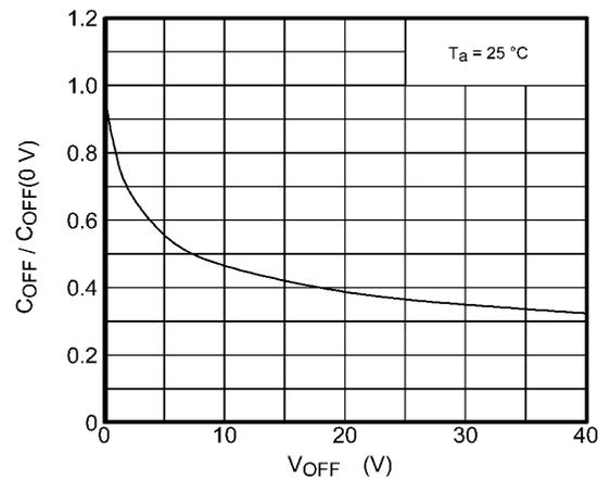
Fig. 12.11  $C_{OFF}/C_{OFF}(0 V) - V_{OFF}$
