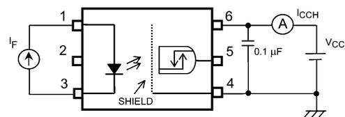
Fig. 13.1.4 ICCCH Test Circuit
