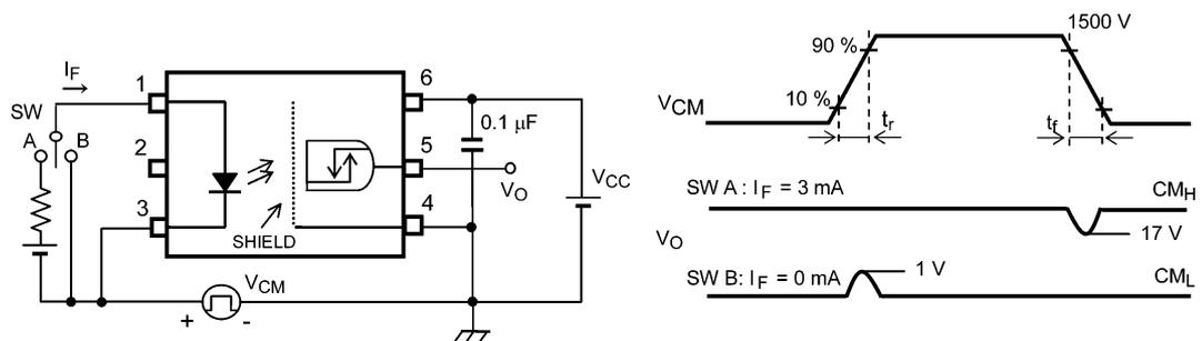
$$CM_L = -\frac{1200 \text{ (V)}}{t_f \text{ (}\mu\text{s)}} \quad CM_H = \frac{1200 \text{ (V)}}{t_r \text{ (}\mu\text{s)}}$$
