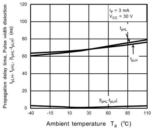
**Fig. 13.2.12  $t_{pLH}, t_{pHL}, |t_{pHL} - t_{pLH}| - T_a$**
