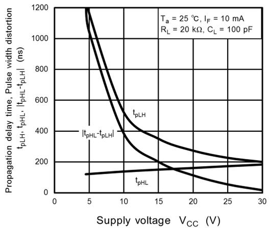
Fig. 13.2.12  $t_{pLH}, t_{pHL}, |t_{pHL} - t_{pLH}| - V_{CC}$
