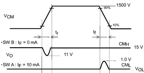
$$CMH = \frac{1200(V)}{t_r(\mu s)} \quad CML = -\frac{1200(V)}{t_f(\mu s)}$$
