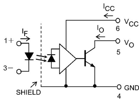
Note: A 0.1- $\mu$ F bypass capacitor must be connected between pin 6 and pin 4.
