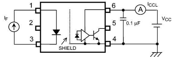
Fig. 13.1.4  $I_{CCL}$  Test Circuit
