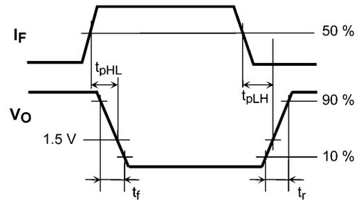
Fig. 13.1.5 Switching Time Test Circuit and Waveform
