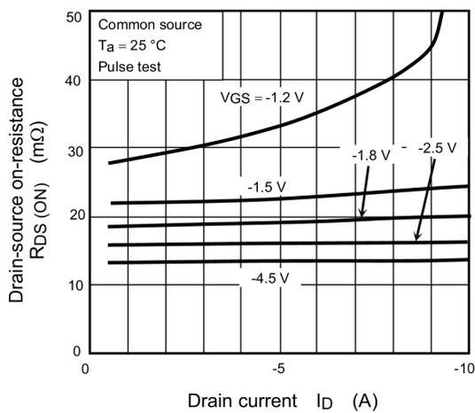
Fig. 7.5  $R_{DS(ON)} - I_D$
