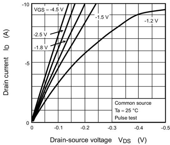
Fig. 7.1  $I_D - V_{DS}$
