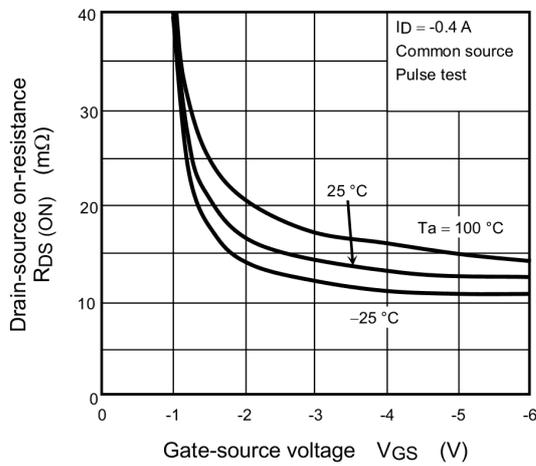
Fig. 7.3  $R_{DS(ON)} - V_{GS}$
