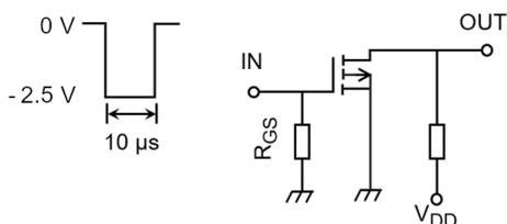
Fig. 5.3.1 Test Circuit of Switching Time
