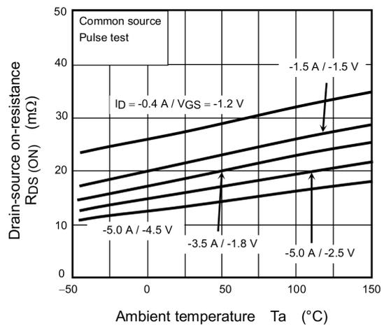
Fig. 7.6  $R_{DS(ON)} - T_a$
