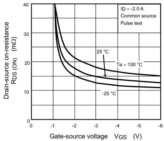
Fig. 7.4  $R_{DS(ON)} - V_{GS}$
