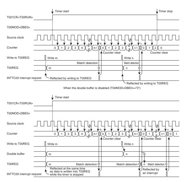
When the double buffer is enabled (T00MOD<DBE0>="1")
