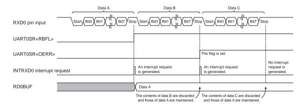
Figure 15-12 Generation of INTRXD0 Interrupt Request
