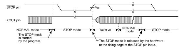
Note: If the rising edge is input to the STOP pin within 1 machine cycle after SYSCR1<STOP> is set to "1", the STOP mode will not be released.
