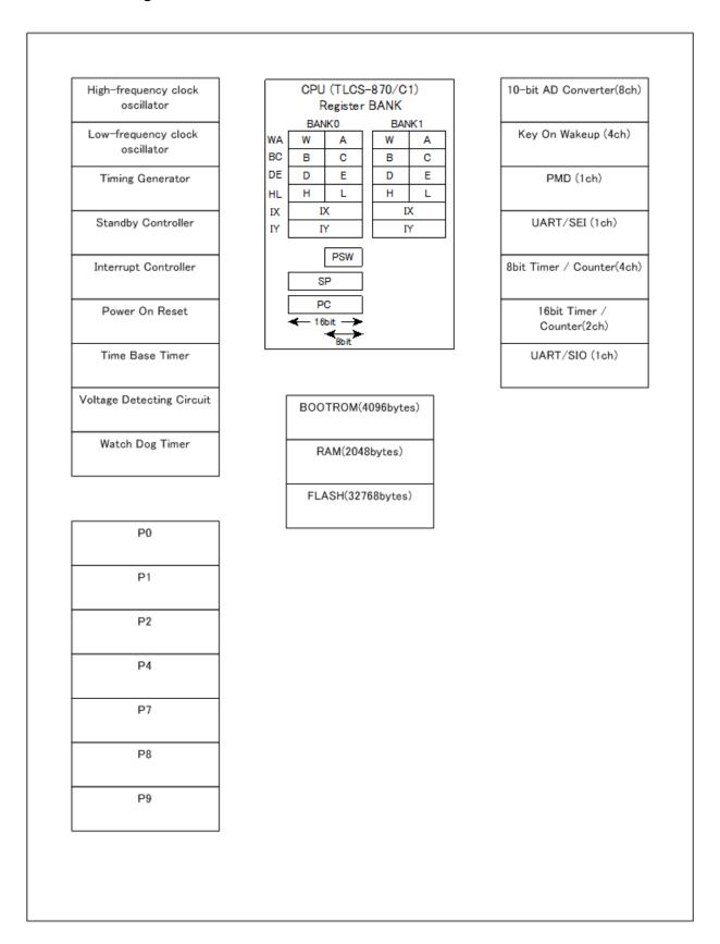
Figure 1-2 Block Diagram
