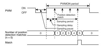
Figure 19-5 Position Detection Sampling Timing with the PWMON Period Selected
