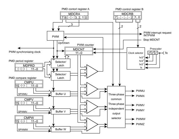
Figure 19-9 Pulse Width Modulation Circuit
