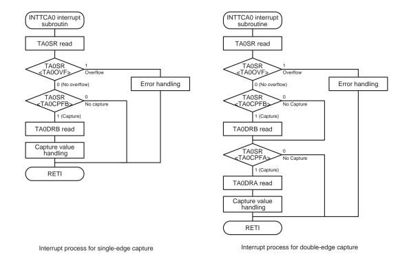
Figure 13-8 Example of capture process
