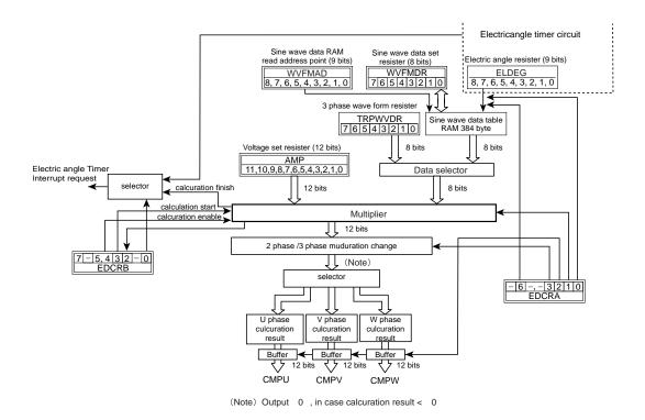
Figure 19-20 Waveform Arithmetic Circuit
