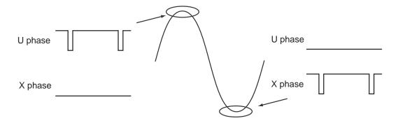
Figure 19-16 How to avoid PWM waveform change
