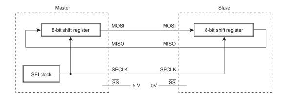
Figure 17-4 Master and Slave Connection in SEI
