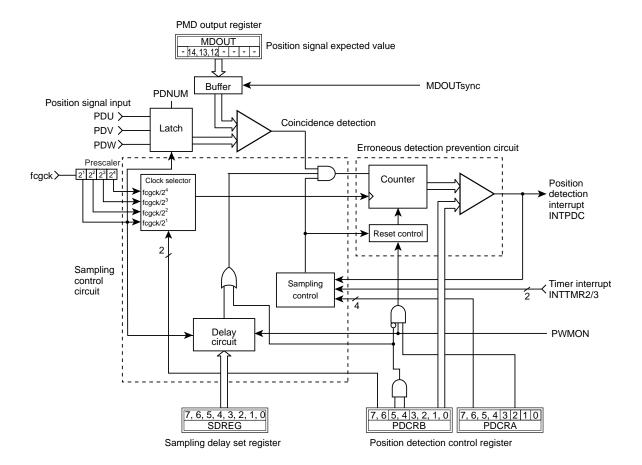
Figure 19-4 Configuration of the Position Detection Circuit
