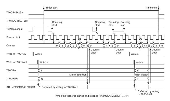
Figure 13-4 External Trigger Timer Timing Chart
