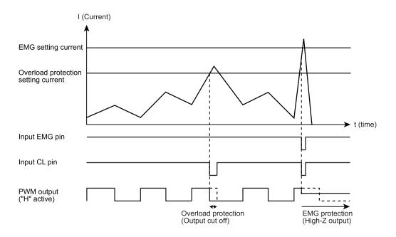
Figure 19-18 Example of Protection Circuit Operation
