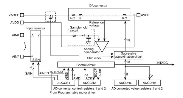
Figure 20-1 10-bit AD Converter
