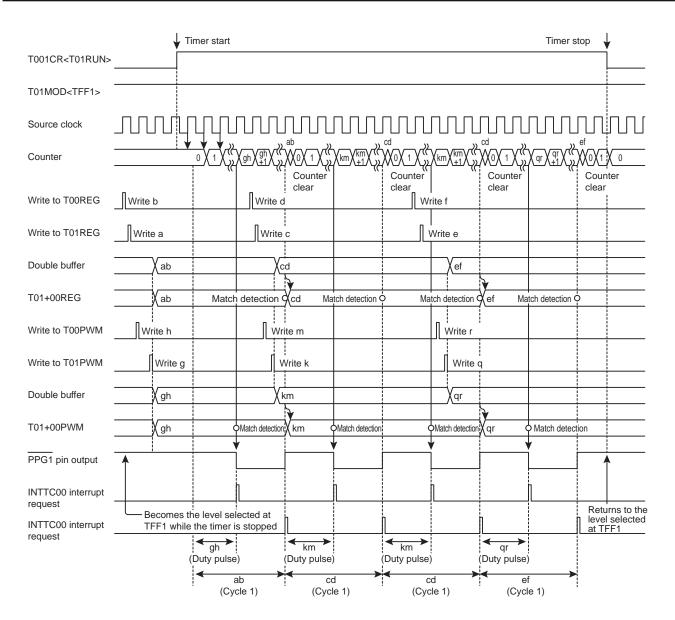
When the double buffer is enabled (T01MOD<DBE1>="1")
