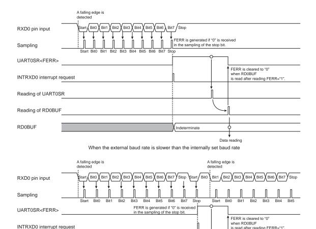
When the external baud rate is faster than the internally set baud rate
