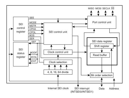
Figure 17-1 SEI (Serial Extended Interface)
