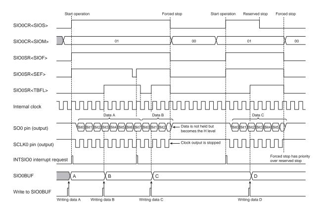
Figure 16-5 8-bit Transmit Mode (Internal Clock and Forced Stop)
