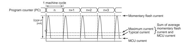
Figure 25-4 Intermittent Operation of Flash Memory
