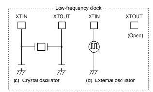
Figure 2-4 Examples of Oscillator Connection
