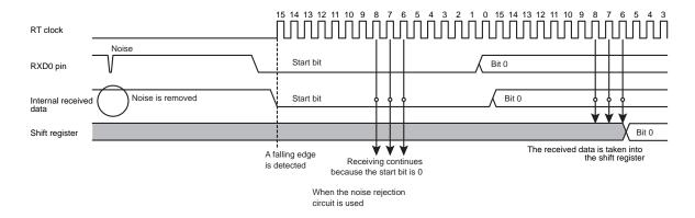
Figure 15-9 Received Data Noise Rejection
