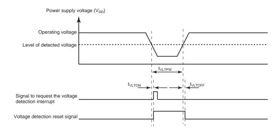
Figure 25-7 Operation Timing of the Voltage Detecting Circuit
