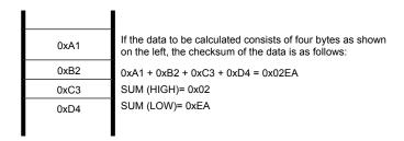
In the case of the product ID code output command and flash memory status output command, however, a different calculation method is used. For more information, refer to Table 22-18.
