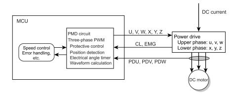
Figure 19-2 Conceptual Diagram of DC Motor Control
