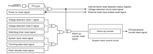
Figure 2-16 Reset Control Circuit
