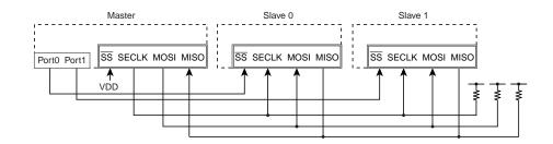
Figure 17-5 Example of SEI System Configuration (1 Master, 2 Slaves)
