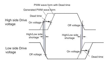
Figure 19-14 PWM waveform with Dead time
