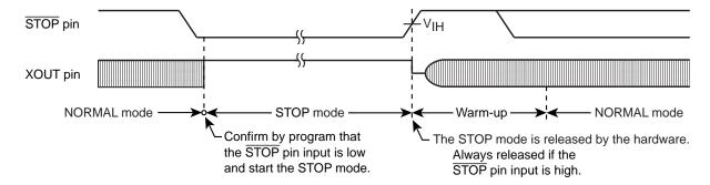
Note: Even if the STOP pin input returns to low after the warm-up starts, the STOP mode is not restarted.
