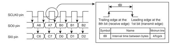
Figure 16-18 Interval time between bytes
