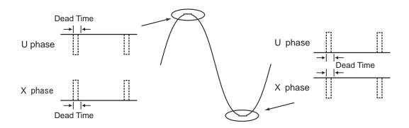
Figure 19-15 Change the shape of PWM waveform
