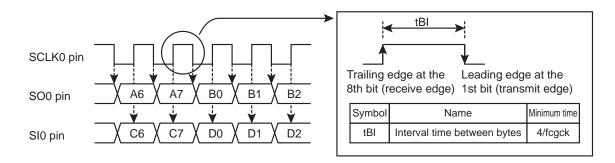
Figure 16-3 Interval time between bytes
