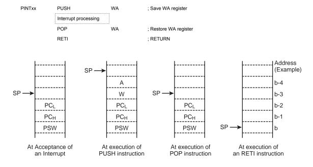
Figure 3-3 Saving/restoring general-purpose registers
