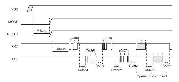
Figure 22-6 Reset Timing
