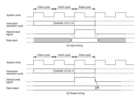
Figure 8-1 Input/Output Timing (Example)
