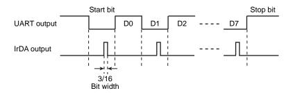
Figure 15-3 Example of Infrared Data Format (Comparison between Normal Output and IrDA Output)
