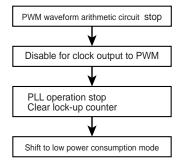
Figure 2-8 The control flow of PLL stop
