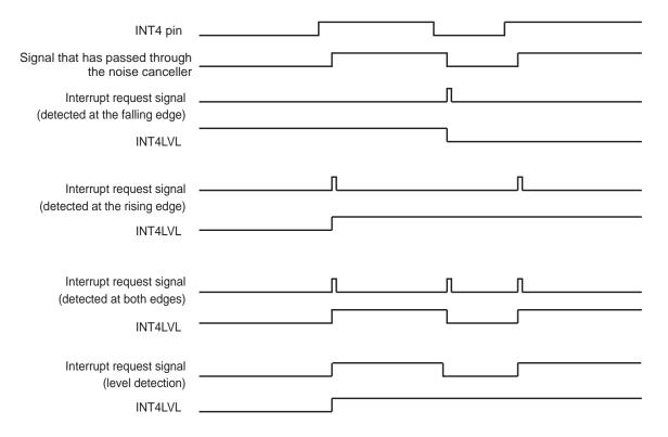
Figure 4-6 Interrupt Request Generation and EINTCR4<INT4LVL>
