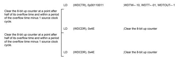
Note: If the overflow of the 8-bit up counter and writing of 0x4E (clear code) into WDCDR occur simultaneously, the 8-bit up counter is cleared preferentially and the overflow detection is not executed.
