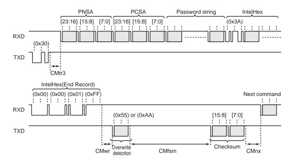
Figure 22-8 Flash Memory Write Command
