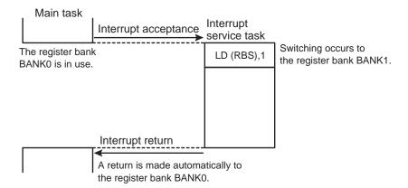
Figure 3-5 Saving/Restoring General-purpose Registers under Interrupt Processing
