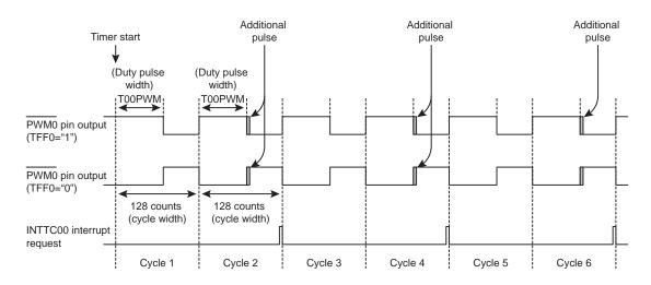
Figure 14-5 PWM0 Pulse Output
