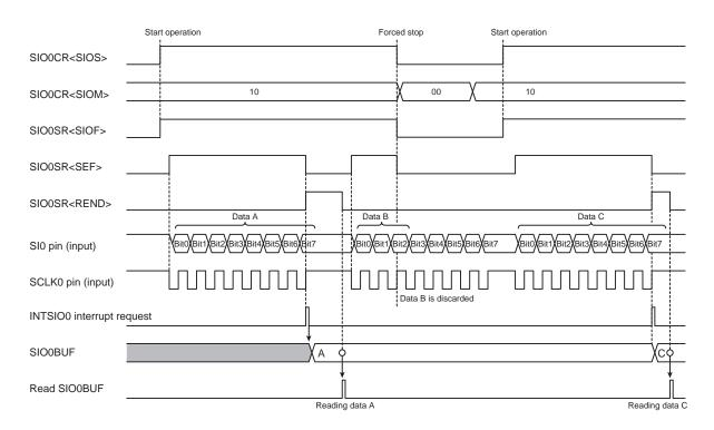
Figure 16-12 8-bit Receive Mode (External Clock and Forced Stop)
