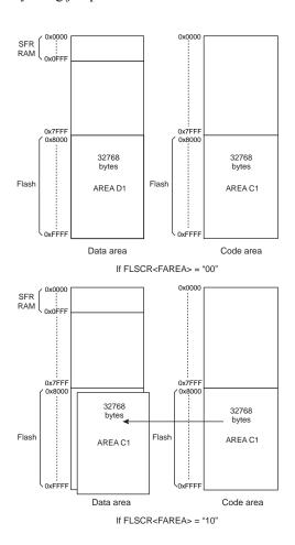
Figure 21-1 Area Switching Using the FLSCR1<FAREA> Setting
