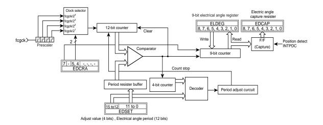
Figure 19-19 Electrical Angle Timer Circuit
