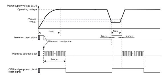
Figure 25-6 Power-on Reset Operation Timing
