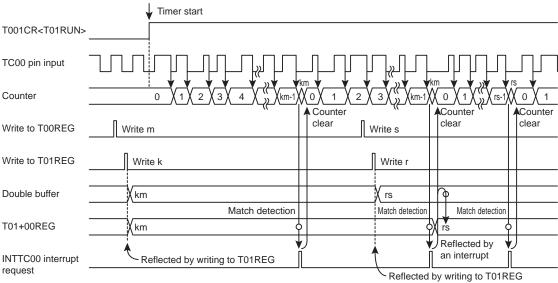
When the double buffer is enabled (T01MOD<DBE1>="1")
