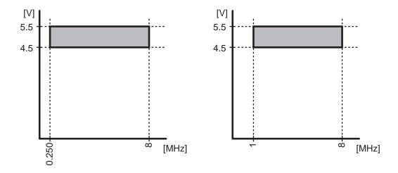
Figure 25-1 Clock gear (fcgck) and High-frequency clock (fc)
