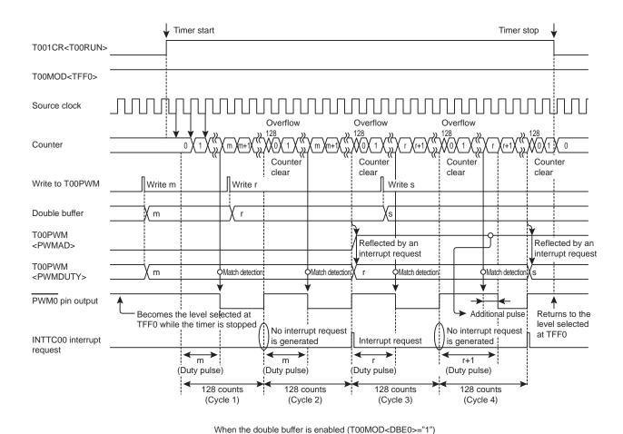
Figure 14-6 8-bit PWM Mode Timing Chart
