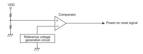
Figure 6-1 Power-on Reset Circuit
