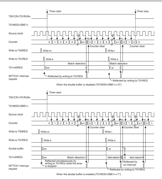
Figure 14-11 16-bit Timer Counter Timing Chart
