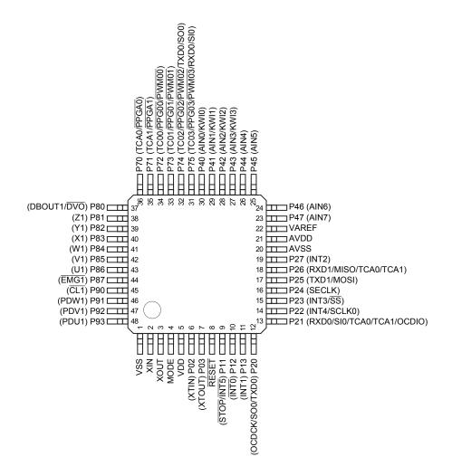
Figure 1-1 Pin Assignment
