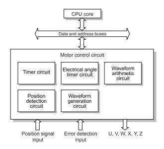
Figure 19-1 Block Diagram of the Motor Control Circuit
