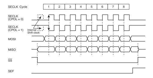
Figure 17-2 Transfer Format When CPHA = 0
