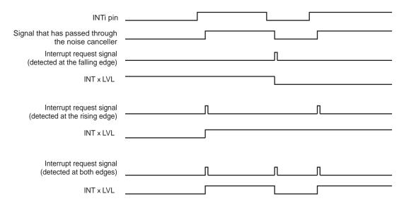
Note: The contents of EINTCRx<INTxLVL> are updated each time an interrupt request signal is generated.
