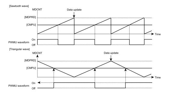
Figure 19-10 PWM Waveforms
