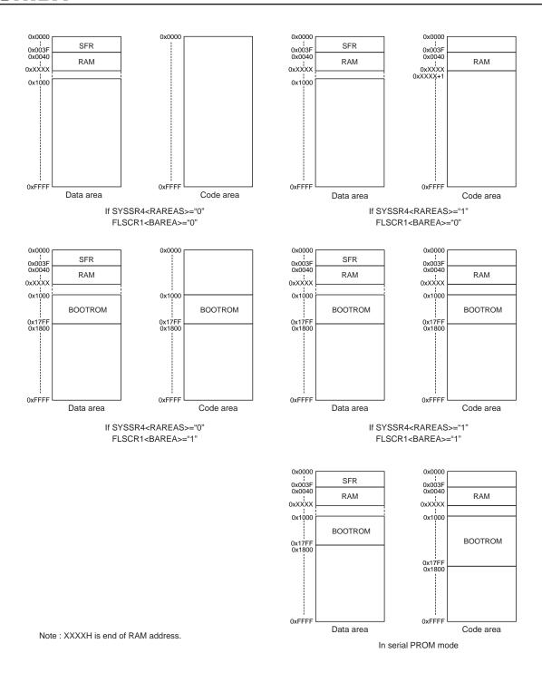
Figure 21-2 Show/Hide Switching for BOOTROM and RAM
