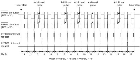
Figure 14-13 Examples of Inserting Additional Pulses
