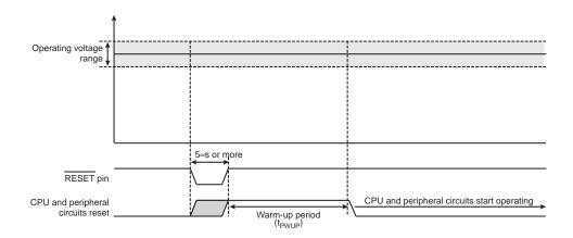
Figure 2-18 External Reset Input (When the Power Supply Is Stable)
