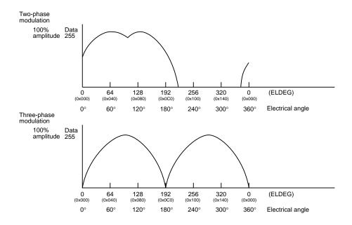
Figure 19-21 Typical Settings of Sine Wave Data
