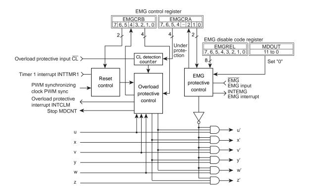
Figure 19-17 Configuration of the Protective Circuit
