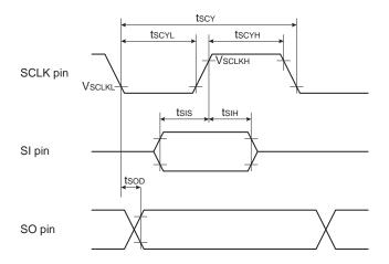
Figure 16-17 AC Characteristics
