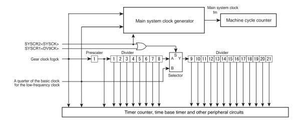
Figure 2-5 Configuration of Timing Generator
