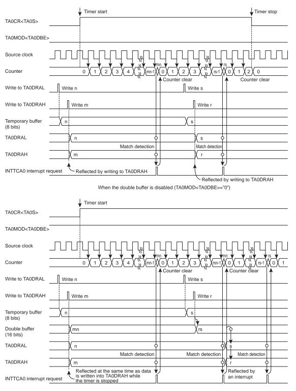
When the double buffer is enabled (TA0MOD<TA0DBE>="1")
