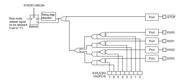
Figure 18-1 Key-on Wakeup Circuit
