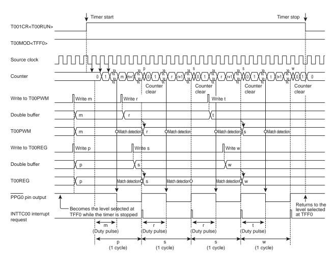
When the double buffer is enabled (T00MOD<DBE0>="1")
