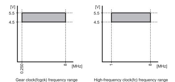
Figure 25-2 Clock gear (fcgck) and High-frequency clock (fc)
