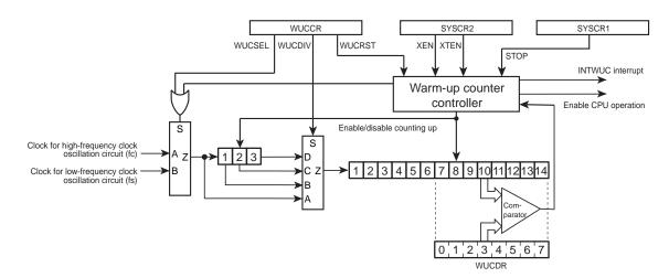
Figure 2-6 Warm-up Counter Circuit
