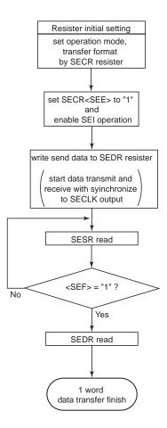
Note: <SEF> is cleared by SEDR resister read or write. Therefore, the SEDR read can omit in case of continuous data transfer.
