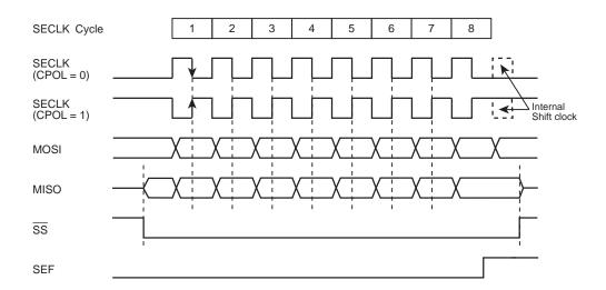
Figure 17-3 Transfer Format When CPHA = 1
