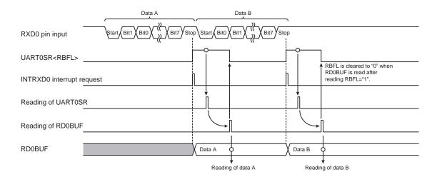
Figure 15-15 Occurrence of Receive Data Buffer Full
