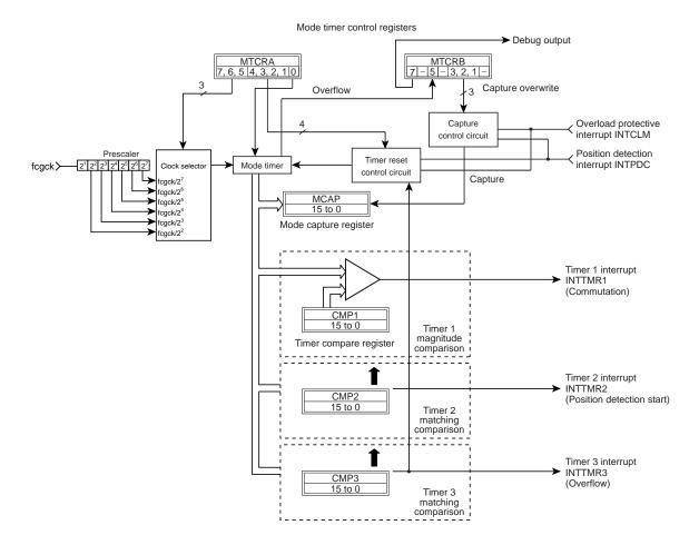
Figure 19-7 Timer Circuit Configuration
