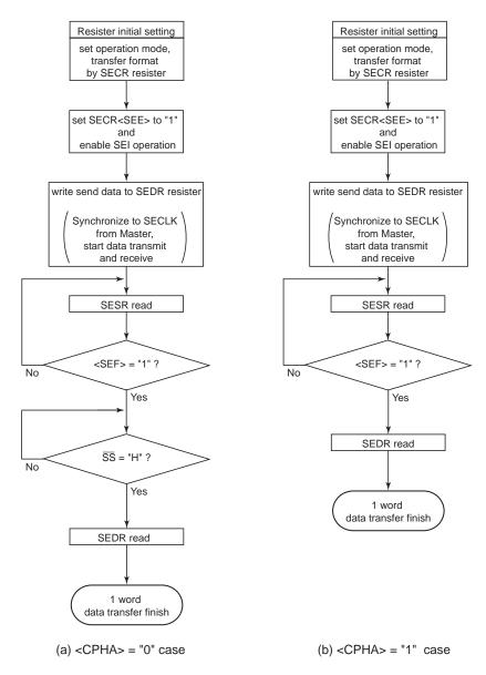
Note 1: <SEF> is cleared by SEDR resister read and write. Therefore, the SEDR read can omit in case of continuous data transfer.
