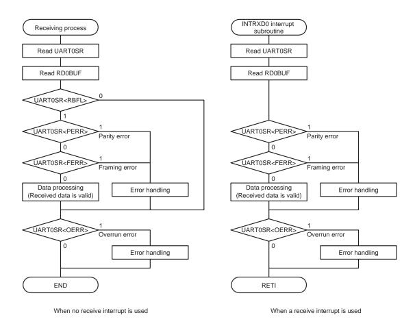
Figure 15-18 Example of Receiving Process
