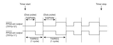
Figure 14-8 PPG0 Pulse Output
