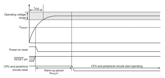
When the supply voltage rises rapidly (When the reset time depends on power-on reset)
