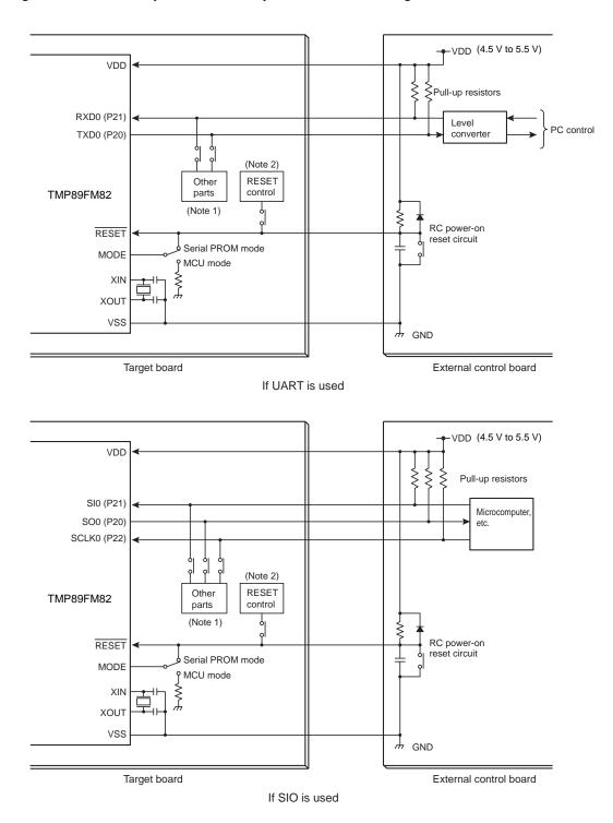
Figure 22-2 Example Connections for On-board Writing
