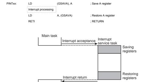
Figure 3-4 Saving/Restoring General-purpose Registers under Interrupt Processing
