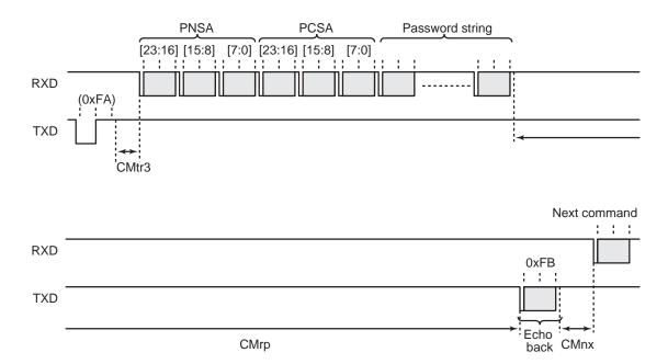
Figure 22-15 Flash Memory Security Setting Command
