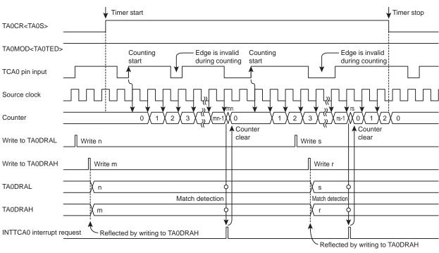
When the trigger is started (TA0MOD<TA0METT>="0")
