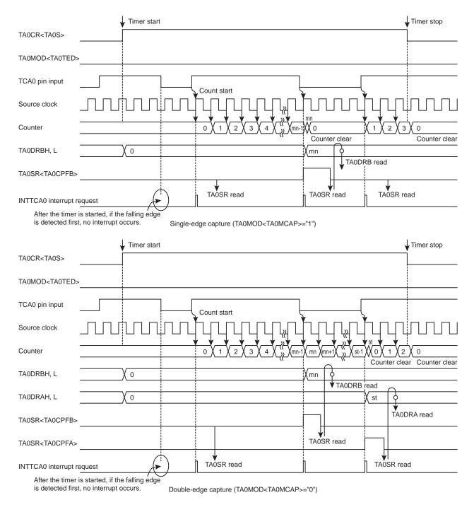
Figure 13-7 Pulse Width Measurement Mode Timing Chart
