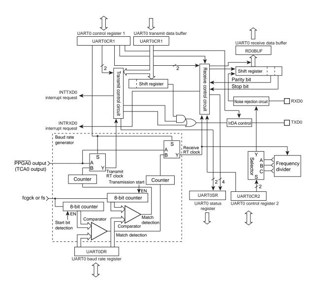
Figure 15-1 Asynchronous Serial Interface (UART)
