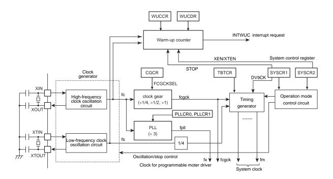
Figure 2-3 System Clock Controller
