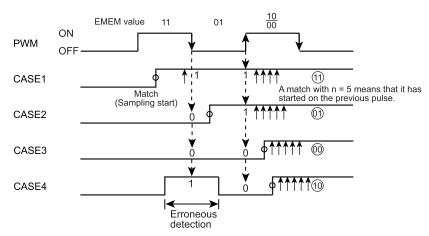
Figure 19-6 Detection Timing of the Position Detection Position
