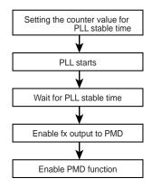
Figure 2-7 The control flow of PLL start
