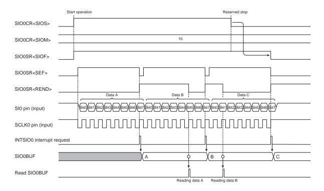
Figure 16-11 8-bit Receive Mode (External Clock and Reserved Stop)
