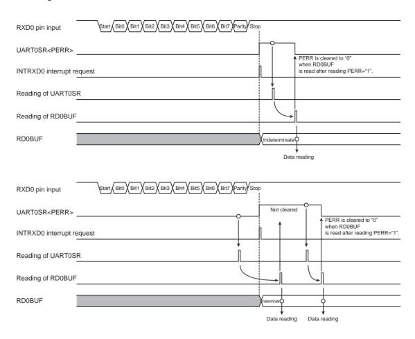
Figure 15-10 Occurrence of Parity Error
