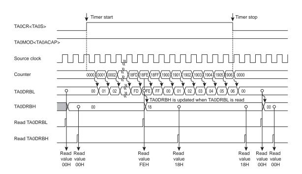
Figure 13-3 Timer Mode Timing Chart (Auto Capture)
