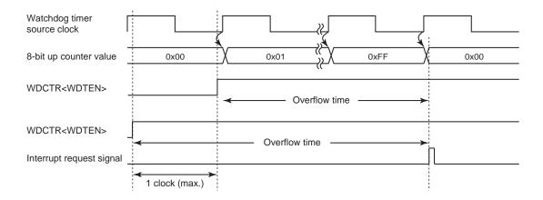
Figure 5-2 WDCTR<WDTEN> Set Timing and Overflow Time
