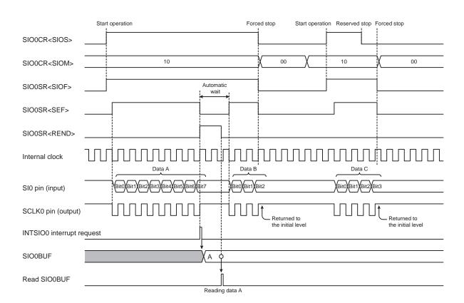
Figure 16-10 8-bit Receive Mode (Internal Clock and Forced Stop)
