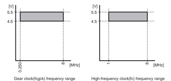
Figure 25-3 Clock gear (fcgck) and High-frequency clock (fc)
