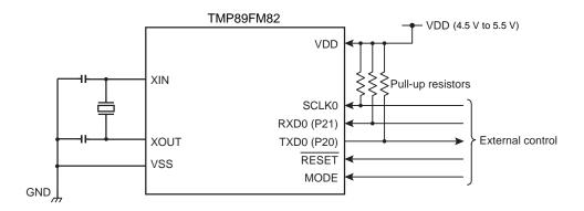
Figure 22-1 Serial PROM Mode Pin Setting
