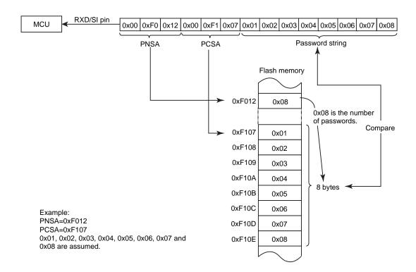
Figure 22-4 Password Structure (Example of a Password Transmitted)
