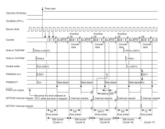
When the double buffer is enabled (T01MOD<DBE1>="1")
