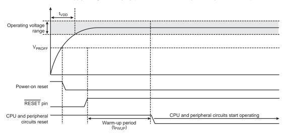
When the supply voltage rises rapidly (When the reset time depends on external reset)
