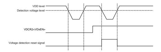
Figure 7-3 Voltage Detection Reset Signal
