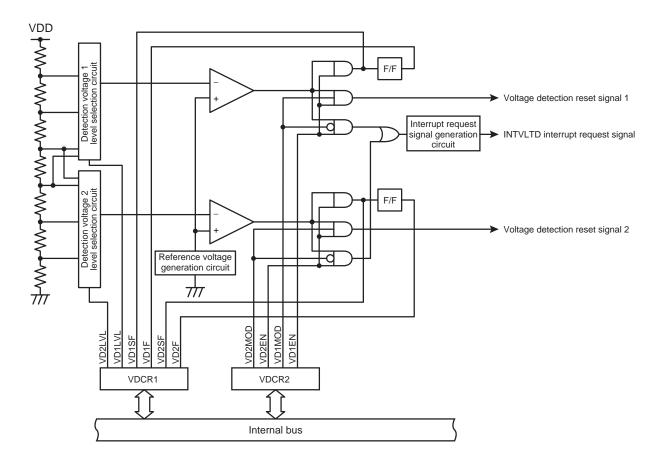
Figure 7-1 Voltage Detection Circuit
