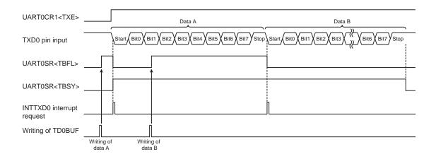
Figure 15-17 Occurrence of Transmit Buffer Full
