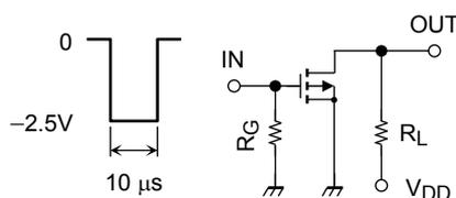
$V_{DD} = -10 \text{ V}$
