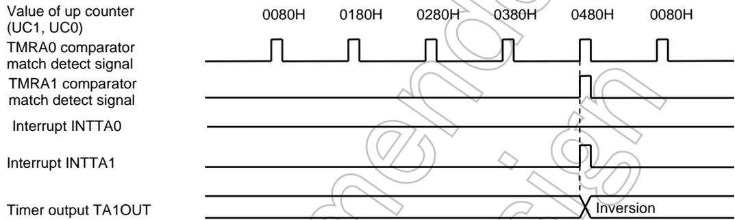
Figure 3.7.12 Timer Output by 16-Bit Timer Mode
