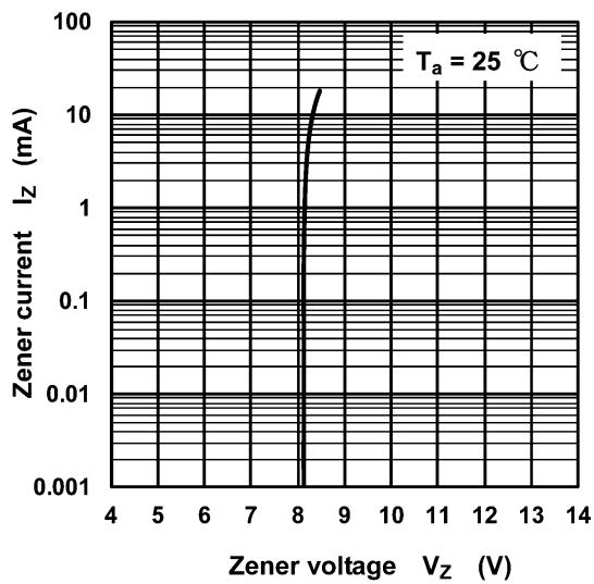
図 8.1  $I_Z - V_Z$
