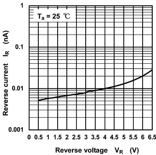
図 8.2  $I_R - V_R$
