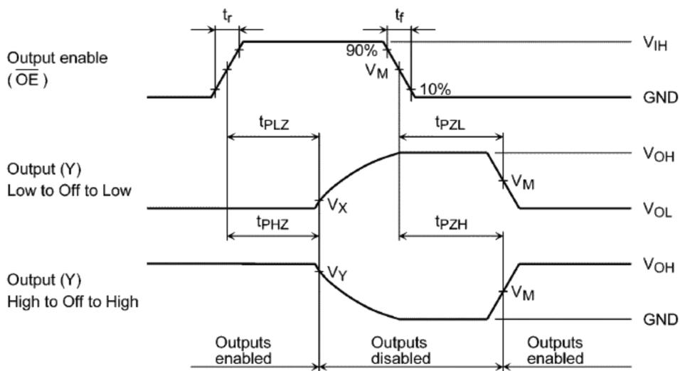
Fig. 11.8.2  $t_{PLZ}$ ,  $t_{PHZ}$ ,  $t_{PZL}$ ,  $t_{PZH}$
