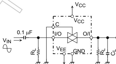
**Figure 4** Feedthrough
