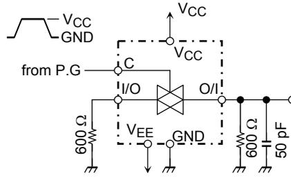
**Figure 5 Cross Talk (control input to output signal)**
