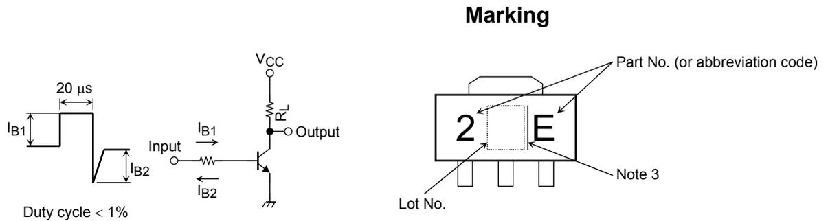
**Figure 1 Switching Time Test Circuit & Timing Chart**
