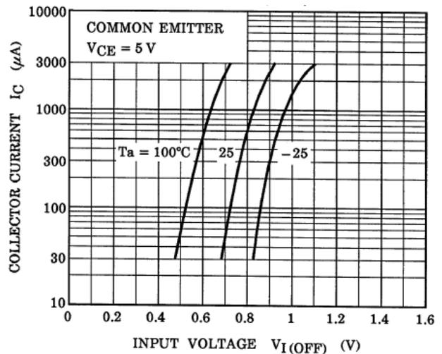
Fig. 10.4 RN1907FE  $I_C$ - $V_{I(OFF)}$
