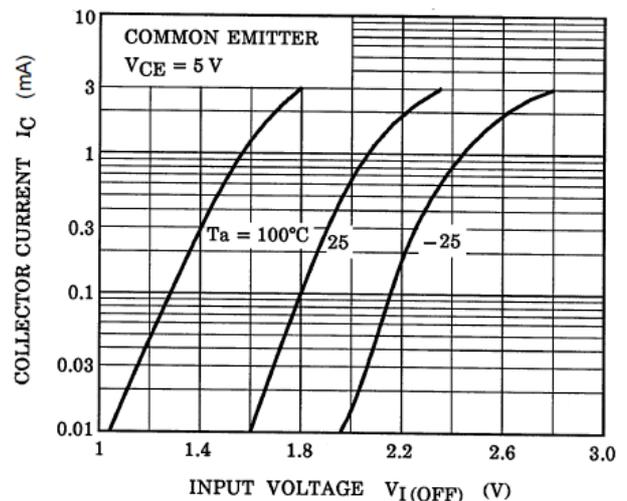
Fig. 10.6 RN1909FE  $I_C$ - $V_{I(OFF)}$
