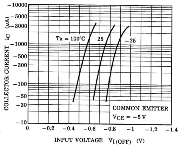
Fig. 10.12 RN2906FE  $I_C$ - $V_{I(OFF)}$
