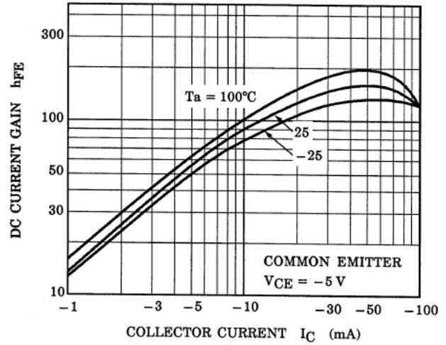
Fig. 10.14 RN2902FE  $h_{FE}$ - $I_C$
