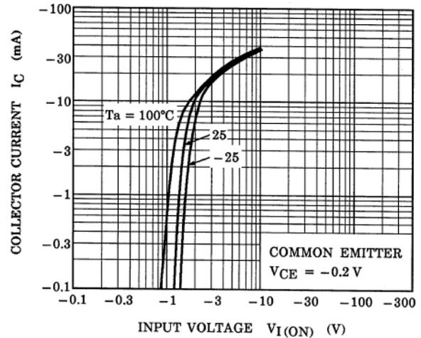
Fig. 10.2 RN2902FE  $I_C$ - $V_{I(ON)}$
