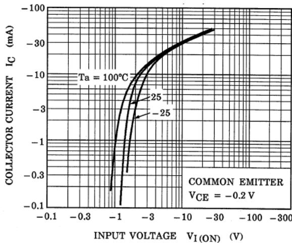
Fig. 10.3 RN2903FE  $I_C$ - $V_{I(ON)}$
