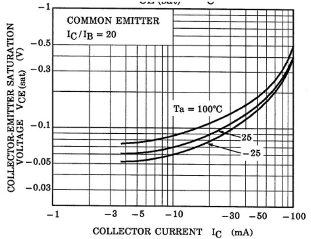
Fig. 10.20 RN2902FE  $V_{CE(sat)}$ - $I_C$
