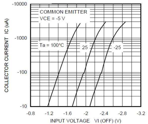
Fig. 10.9 RN2417  $I_C$ - $V_{I(OFF)}$
