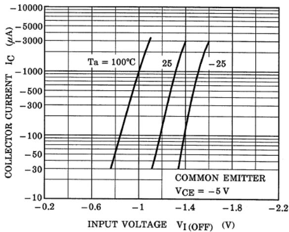
Fig. 10.7 RN2401  $I_C$ - $V_{I(OFF)}$
