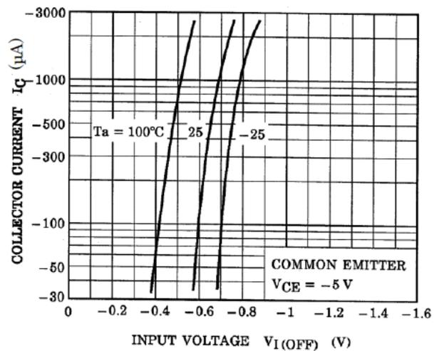
Fig. 9.4 RN2311  $I_C$ - $V_{I(OFF)}$
