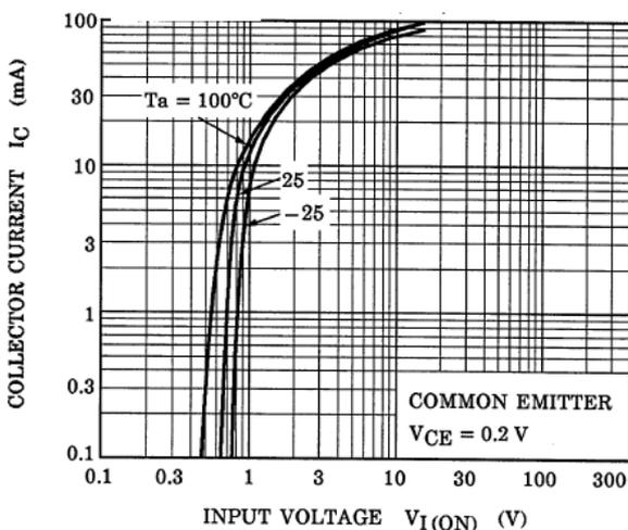
Fig. 10.5 RN1405 I<sub>C</sub>-V<sub>I(ON)</sub>
