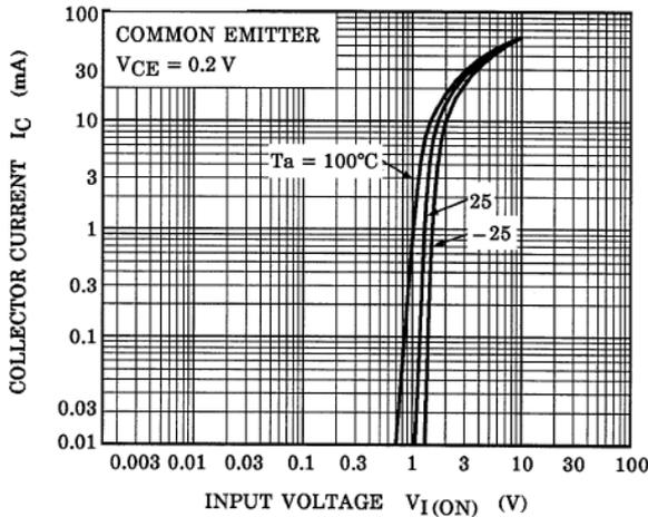
Fig. 10.1 RN1401 I<sub>C</sub>-V<sub>I(ON)</sub>
