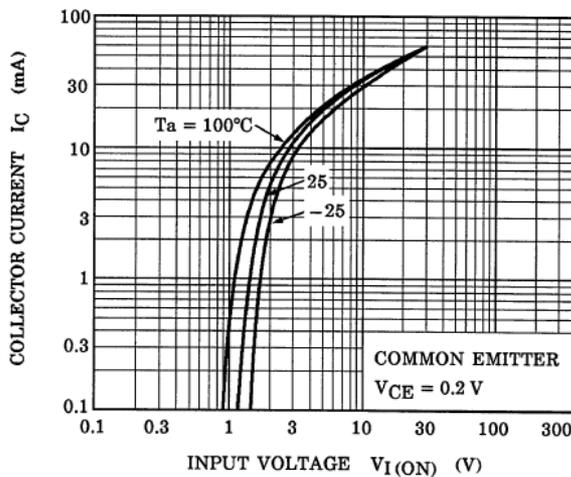
Fig. 10.3 RN1403 I<sub>C</sub>-V<sub>I(ON)</sub>
