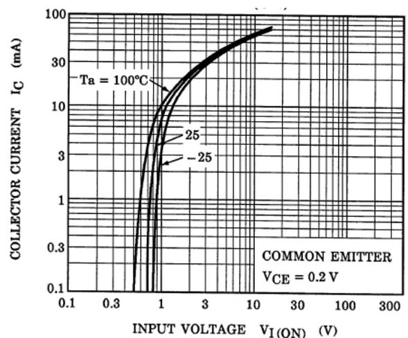
Fig. 10.6 RN1406 I<sub>C</sub>-V<sub>I(ON)</sub>
