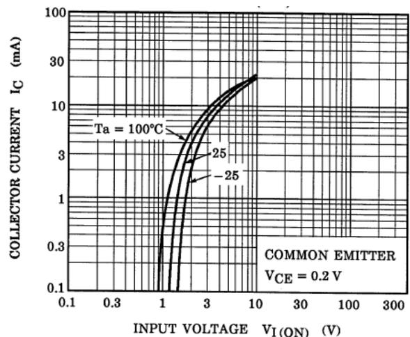
Fig. 10.4 RN1404 I<sub>C</sub>-V<sub>I(ON)</sub>
