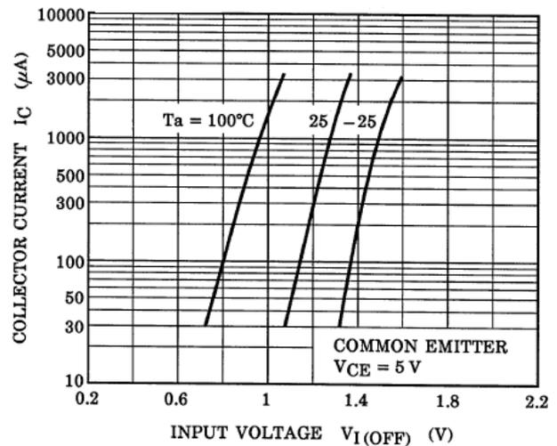
Fig. 10.8 RN1402  $I_C$ - $V_{I(OFF)}$
