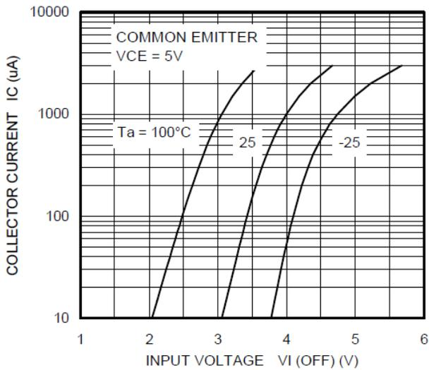
**Fig. 10.10 RN1118  $I_C$ - $V_{I(OFF)}$**
