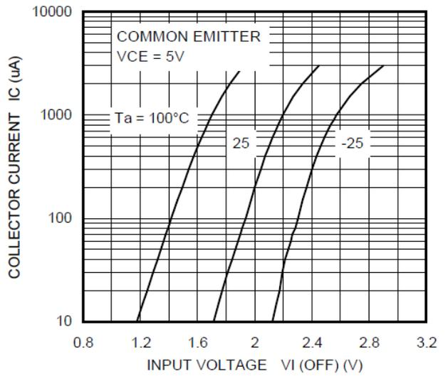
**Fig. 10.9 RN1117  $I_C$ - $V_{I(OFF)}$**
