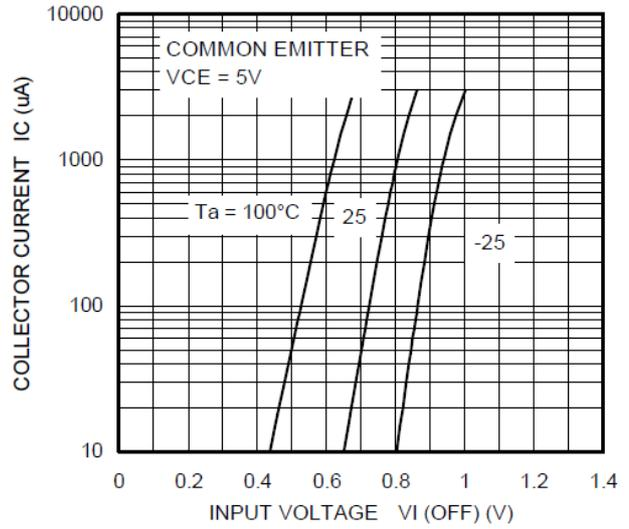
**Fig. 10.7 RN1115  $I_C$ - $V_{I(OFF)}$**
