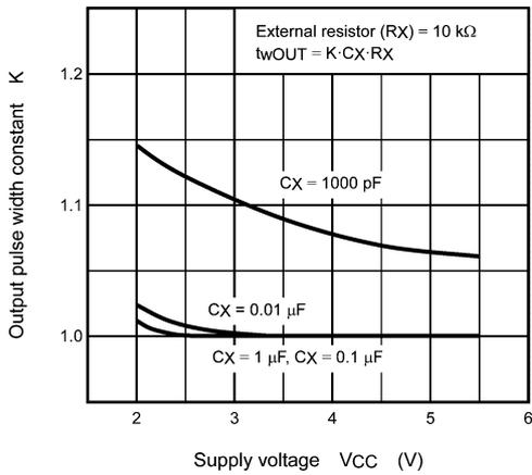
**Fig. 15.3 Output Pulse Width Constant K
