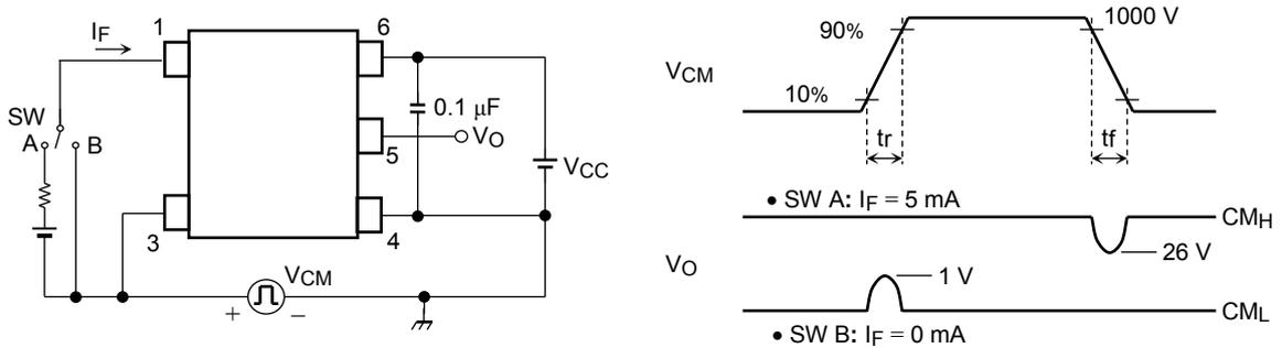
$$C_{ML} = \frac{800 \text{ V}}{t_r (\mu\text{s})}$$
