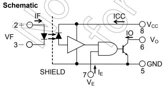
Note: A 0.1µF bypass capacitor must be connected Between pins 8 and 5.
