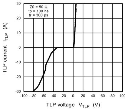
**Fig. 11.20.1**  $I_{TLP} - V_{TLP}$
