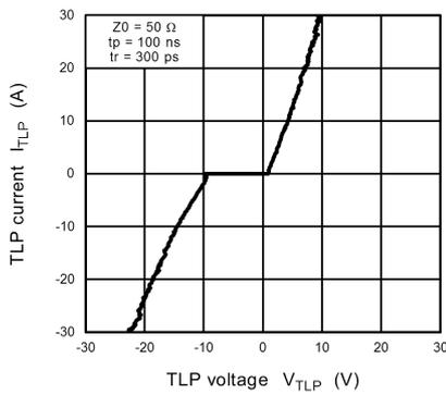
**Fig. 11.8.1  $I_{TLP} - V_{TLP}$**
