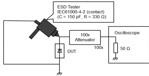
**Fig. 11.22.2 Clamp waveform measurement circuit (according to IEC61000-4-2)**
