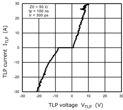
**Fig. 11.6.1  $I_{TLP} - V_{TLP}$**
