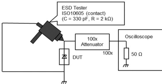
**Fig. 11.22.3 Clamp waveform measurement circuit (according to ISO10605)**
