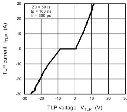
**Fig. 11.7.1  $I_{TLP} - V_{TLP}$**
