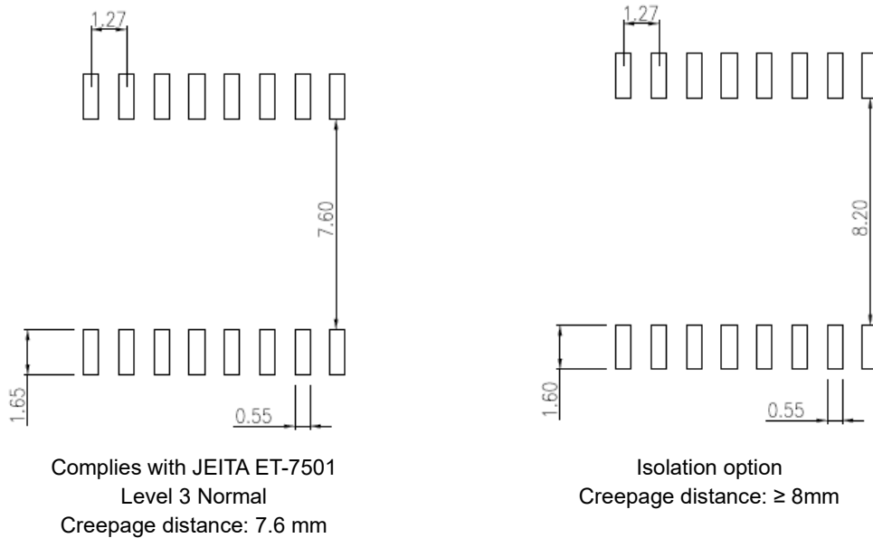
Figure 14.2 Land Pattern Dimensions for Reference only
