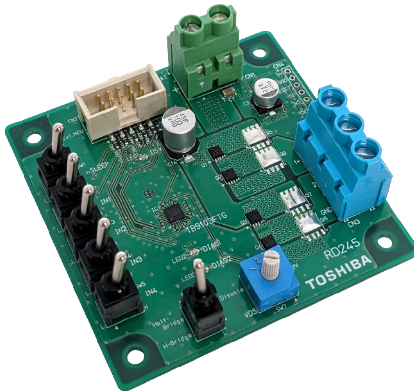
Fig. 2.5 Side View of This Design (with XPN7R104NC MOSFETs)
