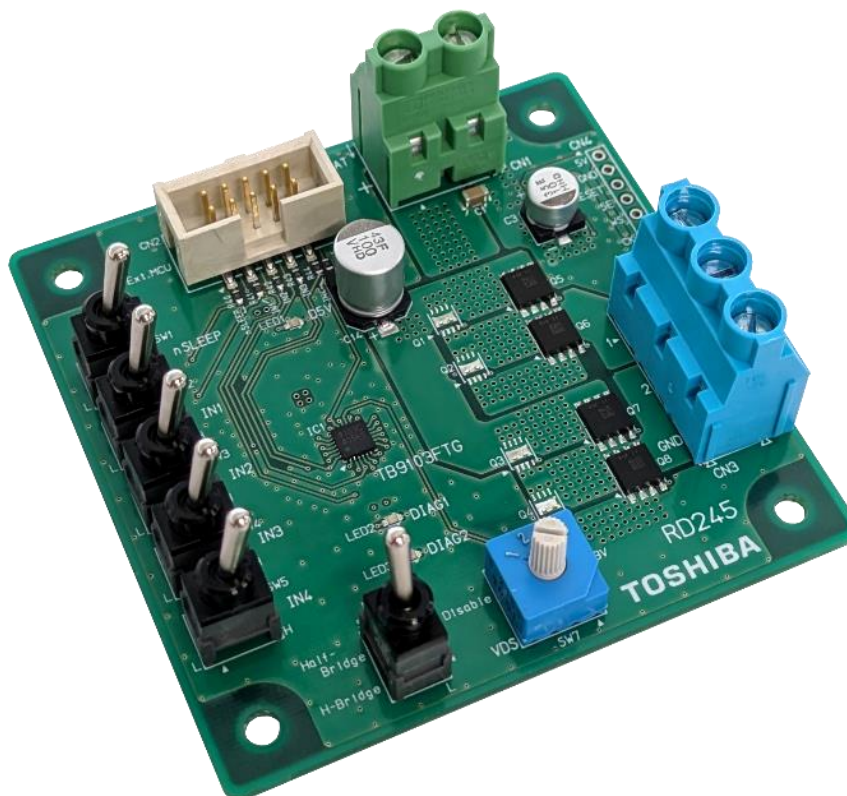
Fig. 2.6 Side View of This Design (with XPH3R304PS MOSFETs)
