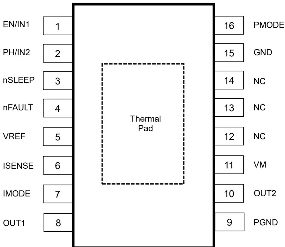
Figure 4.1 TB67S453FNG Pin Assignments (Top view)
