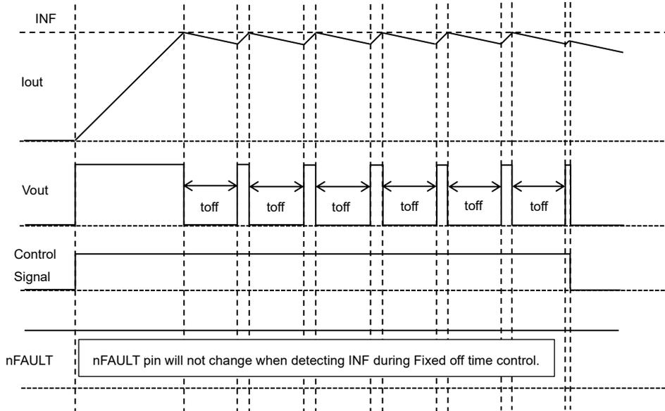
**Figure 7.6 Fixed off time control timing chart example**
