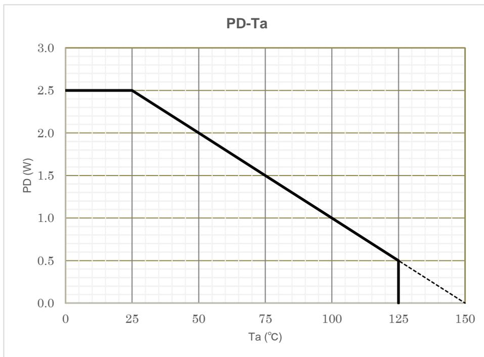
**Figure16 When mounted to a JEDEC 4 layered PCB**
