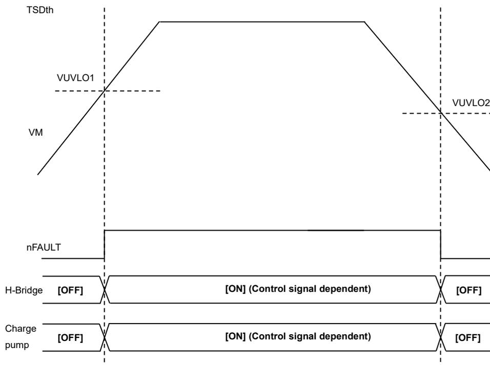
**Figure 8.3 Under voltage lockout timing chart example**
