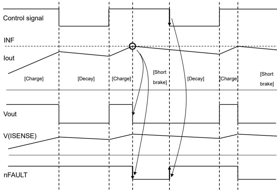
**Figure 7.7.2 Constant current PWM control timing chart example 2**
