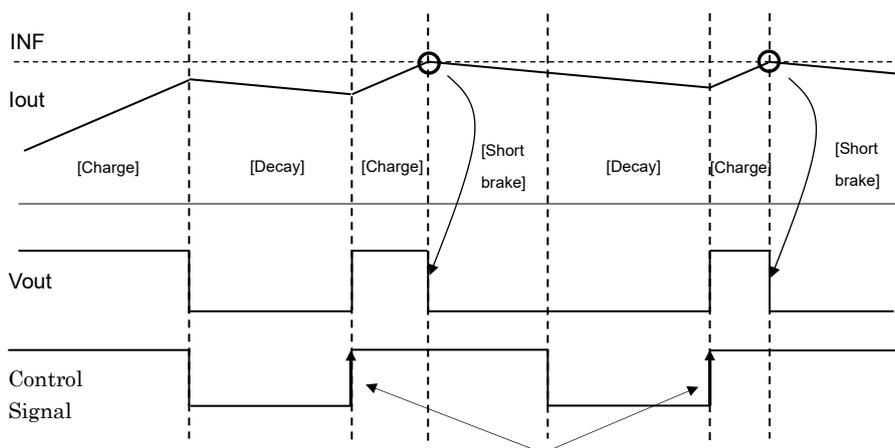
The H-bridge will switch to short brake after the motor current exceeds the current threshold; until the next control signal input edge of EN/IN1 or PH/IN2 is asserted. To reset the outputs after short brake, the next control signal input edge is required.
