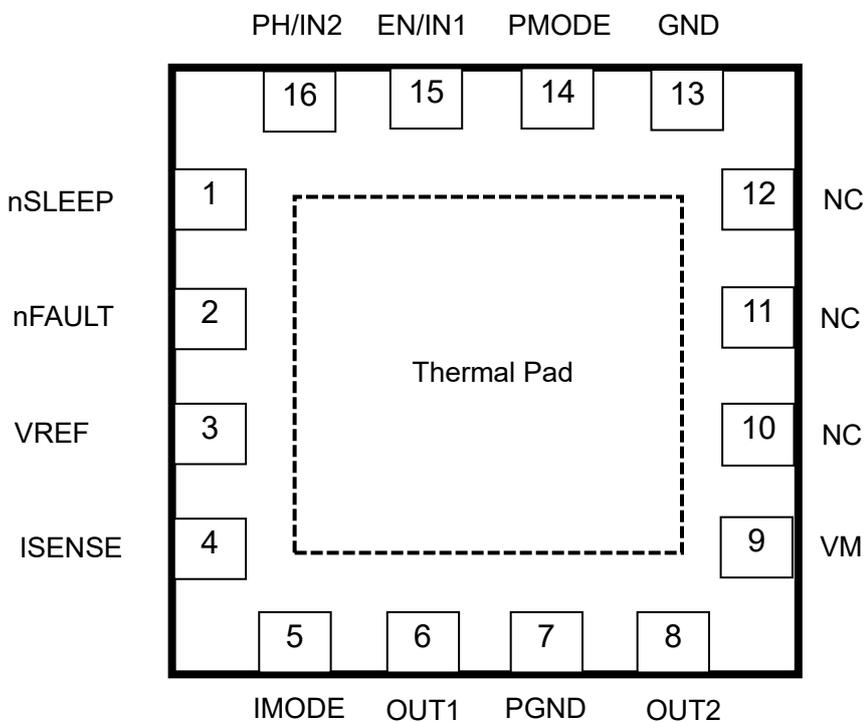
Figure 4.2 TB67H453FTG Pin Assignments (Top view)
