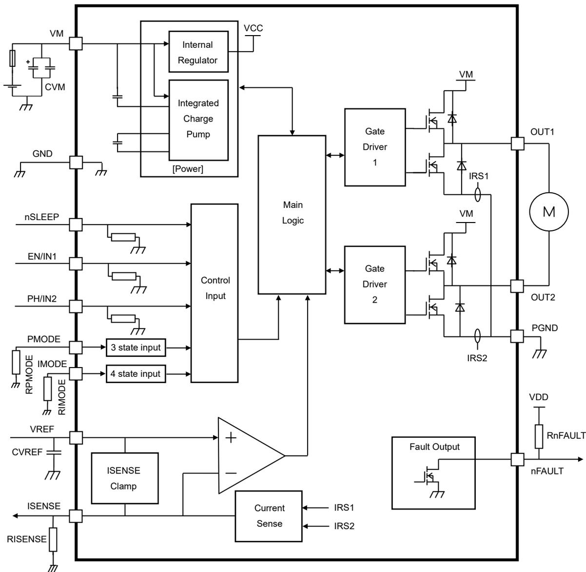
**Figure 17.1 Single brushed DC motor connection example**
