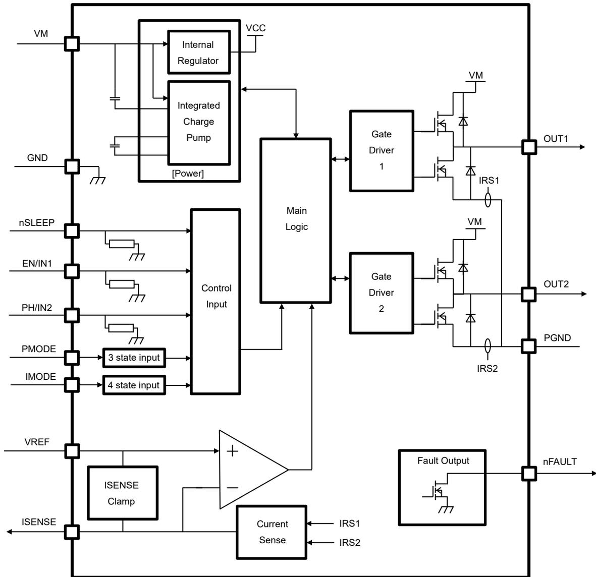
**Figure 3.1 Block Diagram**
