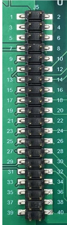
Fig. 4.35 Inverter Circuit Jumper Pin Connector (J5)
