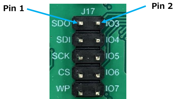
Fig. 4.16 EEPROM connect jumper pin connector (J17)
