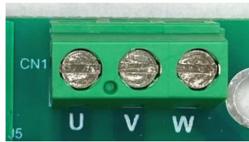
Fig. 4.33 Three-Phase Brushless Motor Terminal (CN1)
