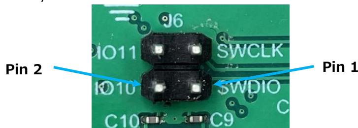
Fig. 4.15 SWD Signal Jumper Pin Connector (J6)
