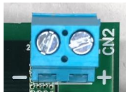
Fig. 4.40 Power Input Pin (CN2)
