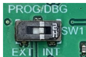
Fig. 4.32 Program/Debug Switch (SW1)
