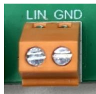
Fig. 4.34 LIN Input/Output Terminal (TB2)
