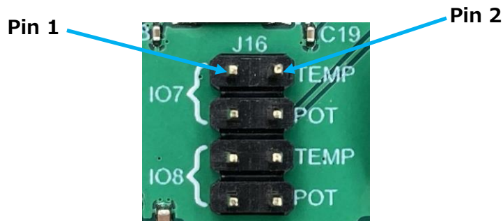
Fig. 4.11 TEMP-POT Signal Jumper Pin Connector (J16)
