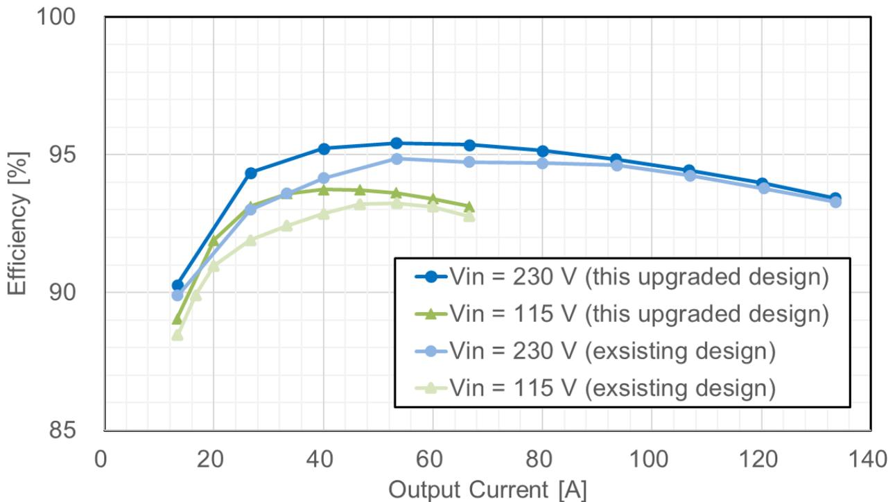
**Fig. 5.1 Efficiency Measurement (When Input is AC 230 V or AC 115 V)**
