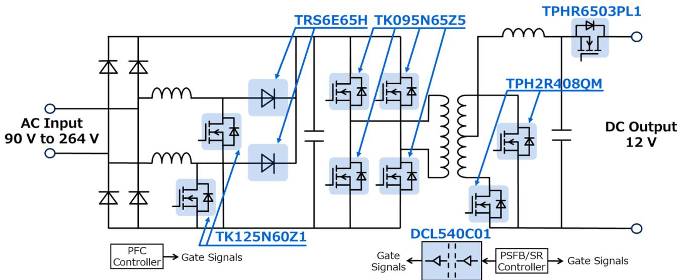
**Fig. 2.1 Block Diagram of the 1.6 kW Server Power Supply (Upgraded)**
