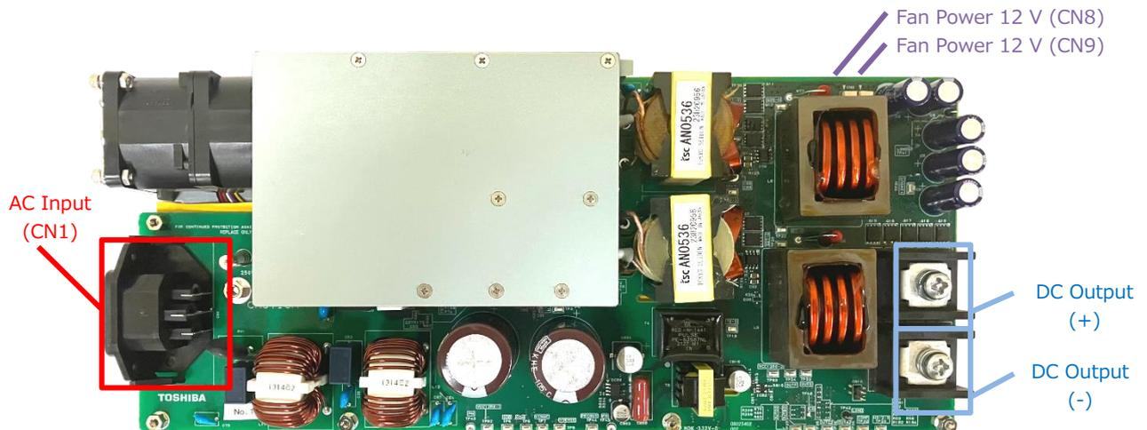
Fig. 4.1 External Connections
