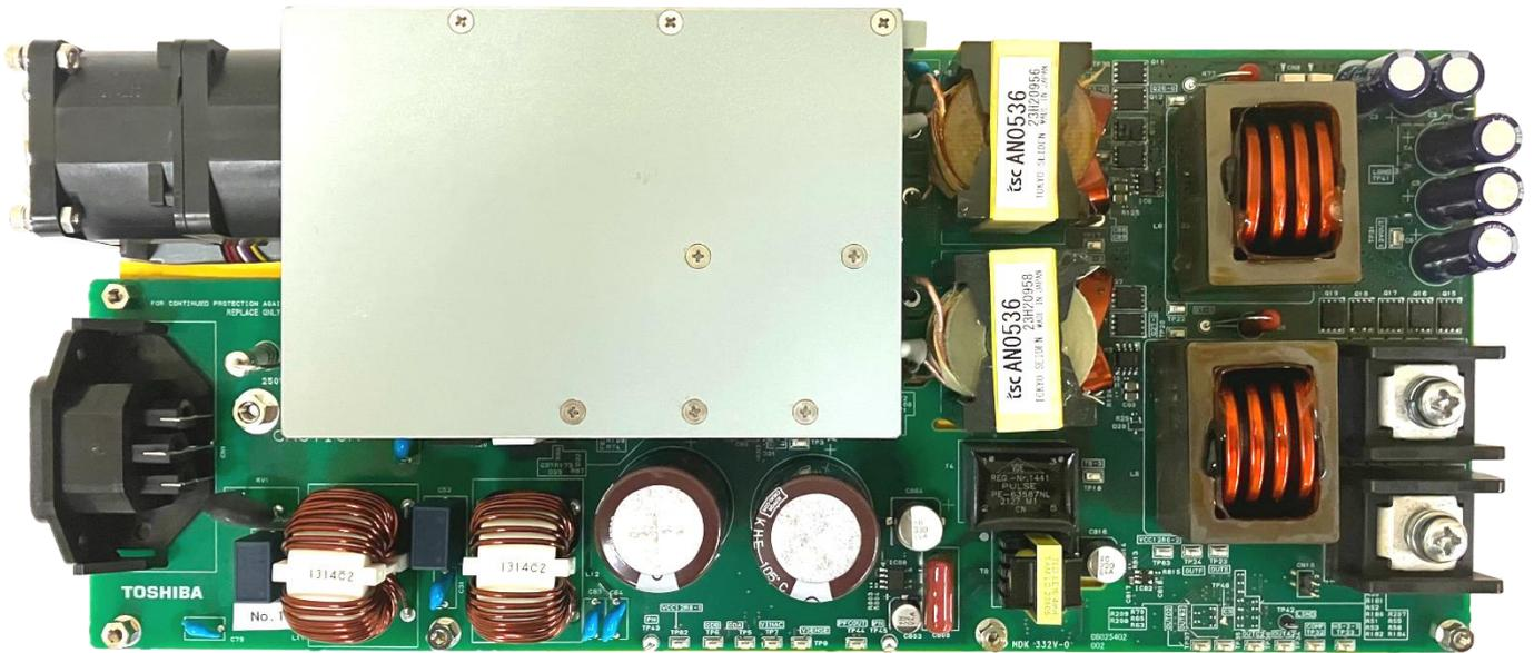
**Fig. 2.3 Front View of the 1.6 kW Server Power Supply (Upgraded)**
