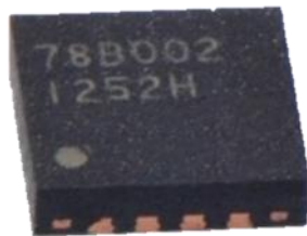
WQFN16 Package (3 x 3 x 0.75 mm)
