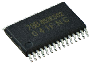
SSOP30-P-300-0.65 Package (10.2 x 7.6 x 1.6 mm)
