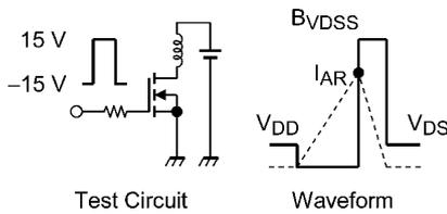
$$R_G = 25 \Omega, V_{DD} = 90 \text{ V} \quad E_{AS} = \frac{1}{2} \cdot L \cdot I_{AR}^2 \cdot \left( \frac{B_{VDSS}}{B_{VDSS} - V_{DD}} \right)$$
