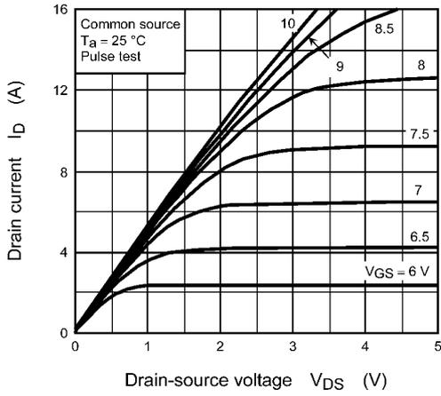
**Fig. 8.1  $I_D - V_{DS}$**
