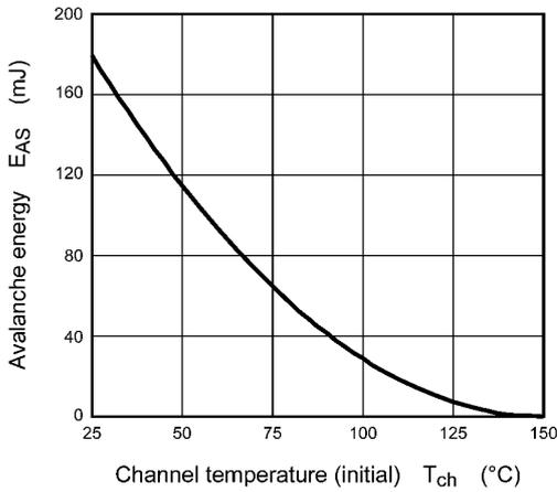
**Fig. 8.14  $E_{AS} - T_{ch}$**
