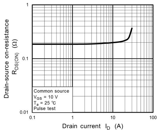
**Fig. 8.6  $R_{DS(ON)} - I_D$**
