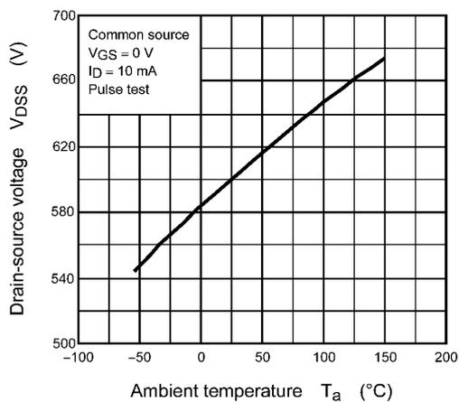
**Fig. 8.5  $V_{DSS} - T_a$**
