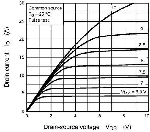
**Fig. 8.2  $I_D - V_{DS}$**
