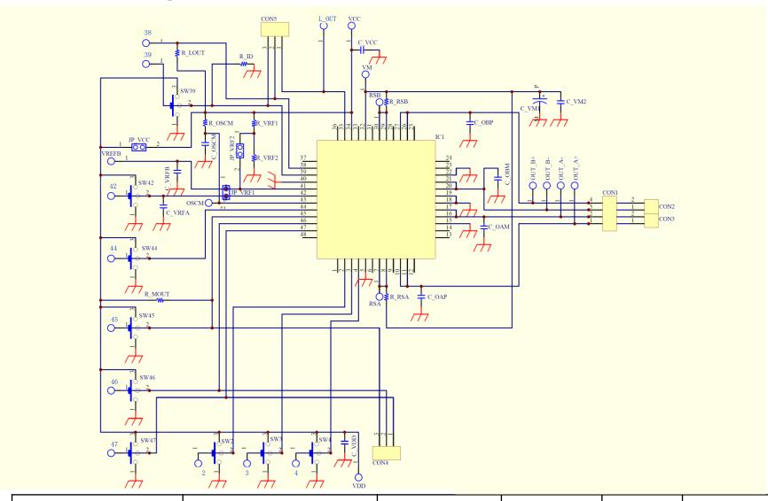
Control Num.TITLEFunctionSheet Num.Rev.DateRD066-SCHEMATIC-02TB67H400AFTG Circuit diagramMotor Driver1/1022018-09-21
