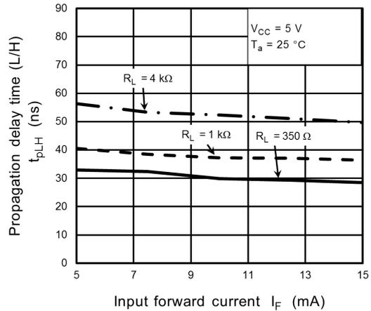
**Fig. 13.2.20**  $t_{pLH} - I_F$
