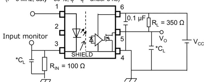
\* $C_L$  is less than 15 pF which includes probe and stay wiring capacitance.
