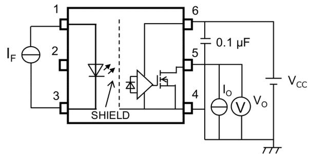
Fig. 13.1.2 VOL Test Circuit
