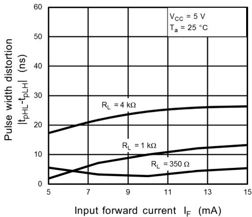
**Fig. 13.2.21**  $|t_{pHL} - t_{pLH}| - I_F$
