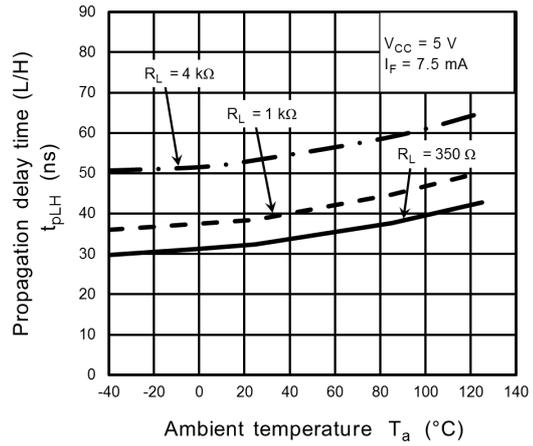
**Fig. 13.2.14**  $t_{pLH} - T_a$
