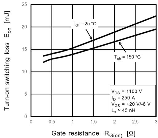
**Fig. 8.10  $E_{on} - R_{G(on)}$**
