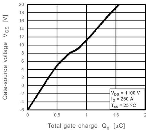
**Fig. 8.5  $V_{GS} - Q_g$**
