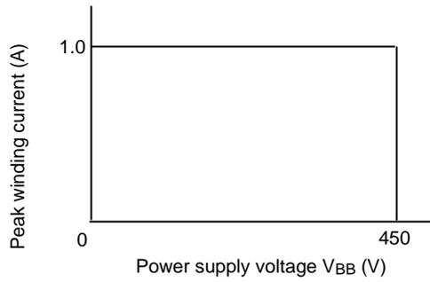
**Figure 11.1 SOA at  $T_j = 135\text{ }^\circ\text{C}$**
