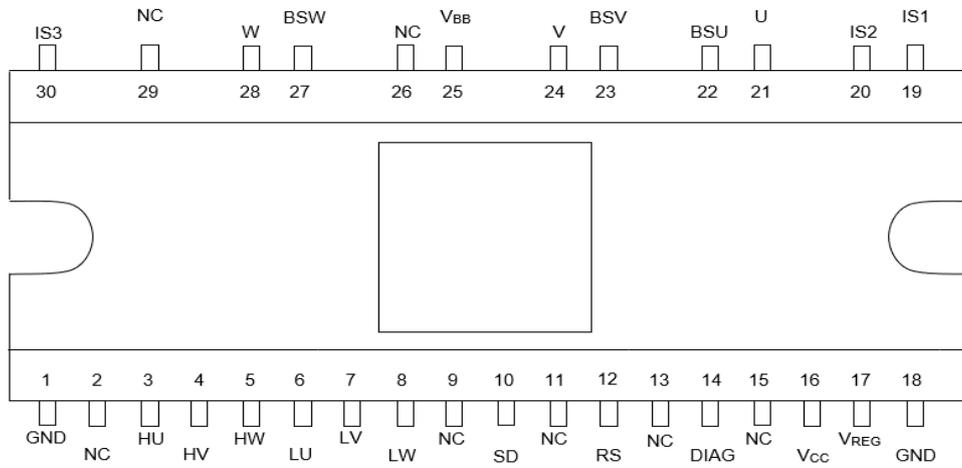
Figure 5.1 Pin Assignments
