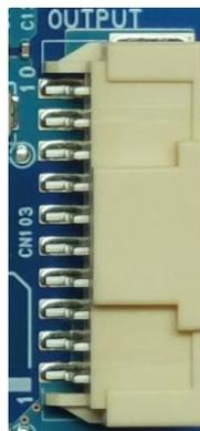
**Fig. 4.2 Power Output Connector**
