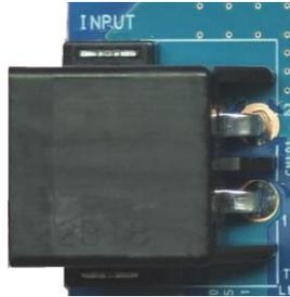
**Fig. 4.1 Power Input Connector**
