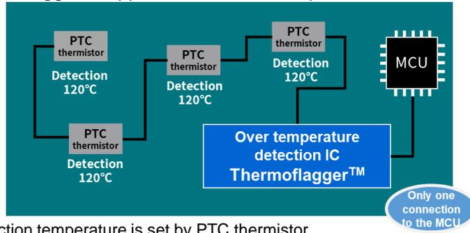
Detection temperature is set by PTC thermistor
