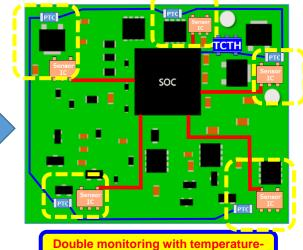
sensor and overheat monitoring IC+PTC
