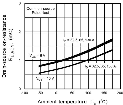
**Fig. 8.9  $R_{DS(ON)} - T_a$**
