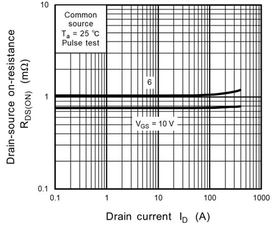
**Fig. 8.8  $R_{DS(ON)} - I_D$**
