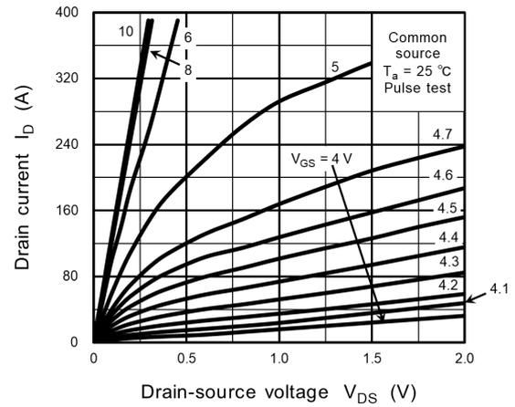
Fig. 8.2  $I_D - V_{DS}$
