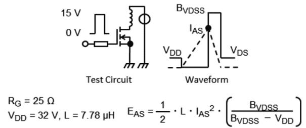
**Fig. 8.16 Test Circuit/Waveform**
