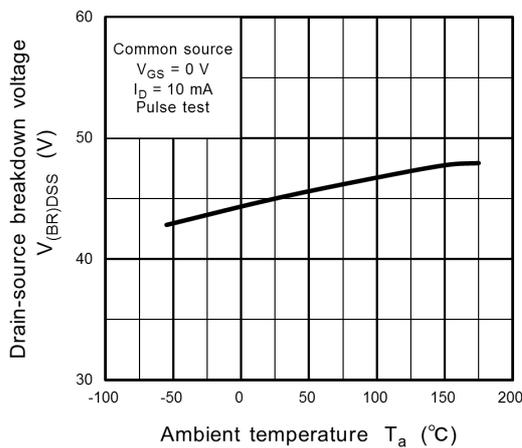
**Fig. 8.11  $V_{(BR)DSS} - T_a$**
