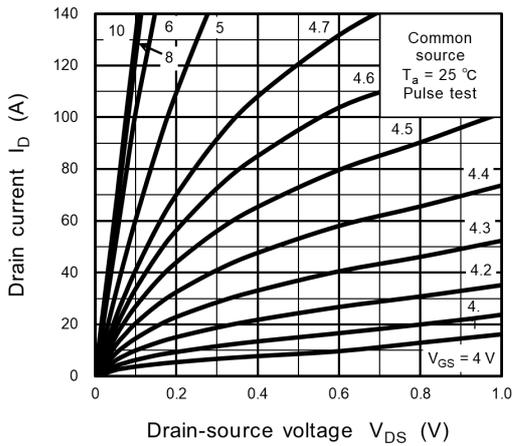
Fig. 8.1  $I_D - V_{DS}$
