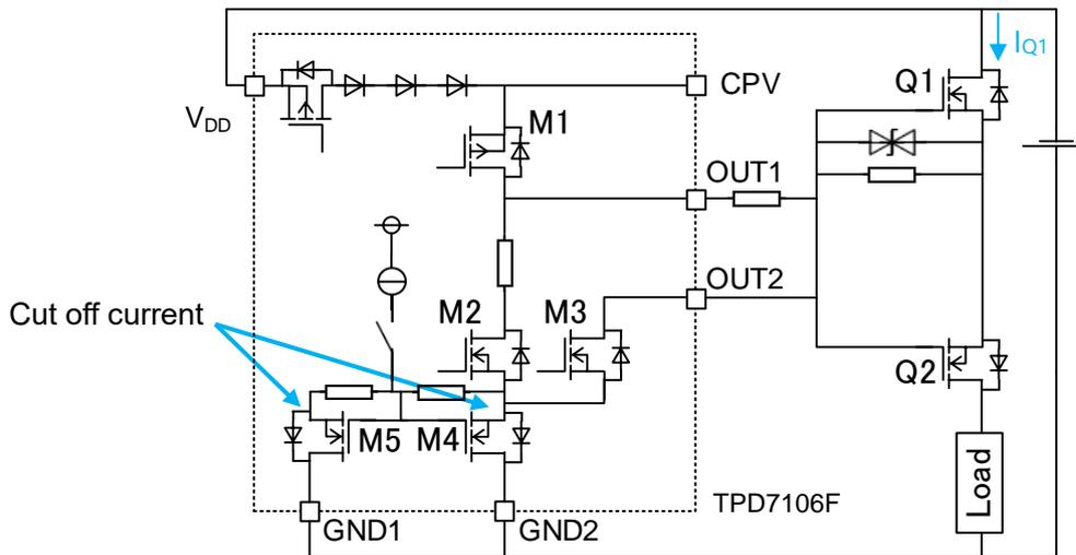
Fig. 2.7 Behavior of power reverse connection
