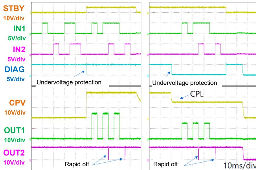
Fig. 2.6 Low voltage detection waveform
