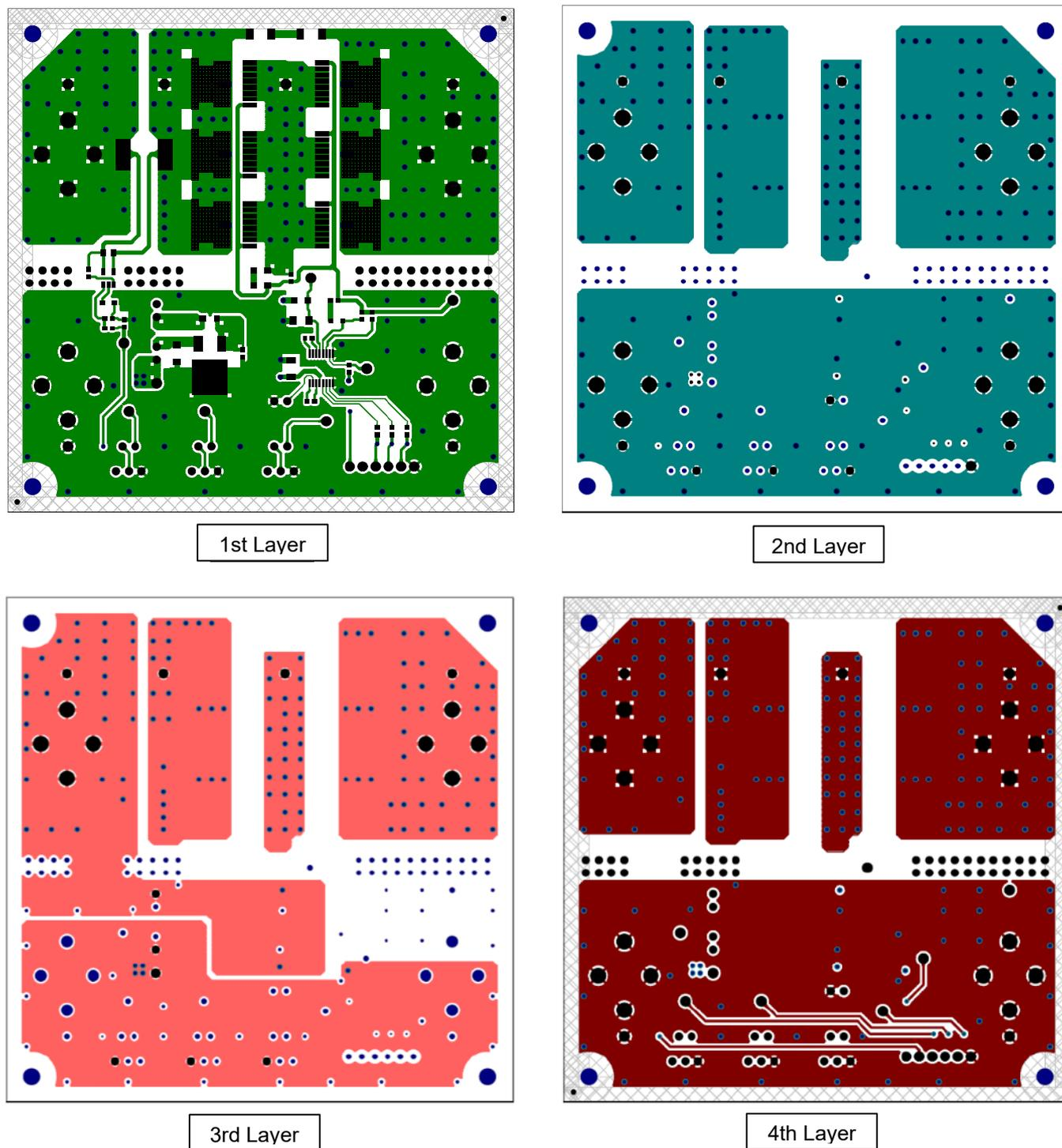
Fig. 7.5 TPD7106F evaluation board layout
