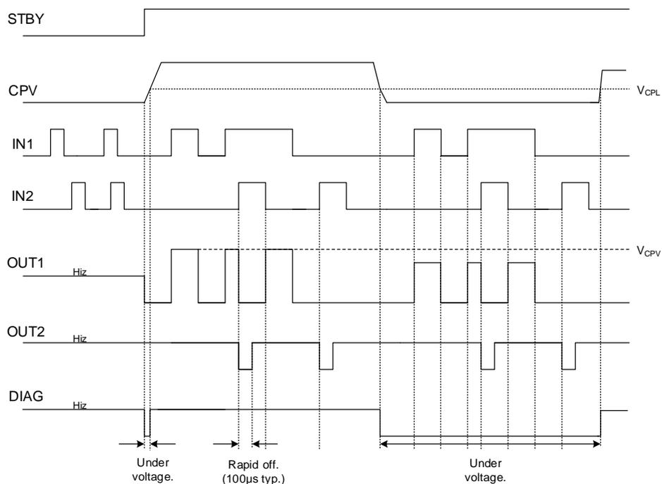
**Fig. 2.5** Low voltage detection function of charge pump voltage
