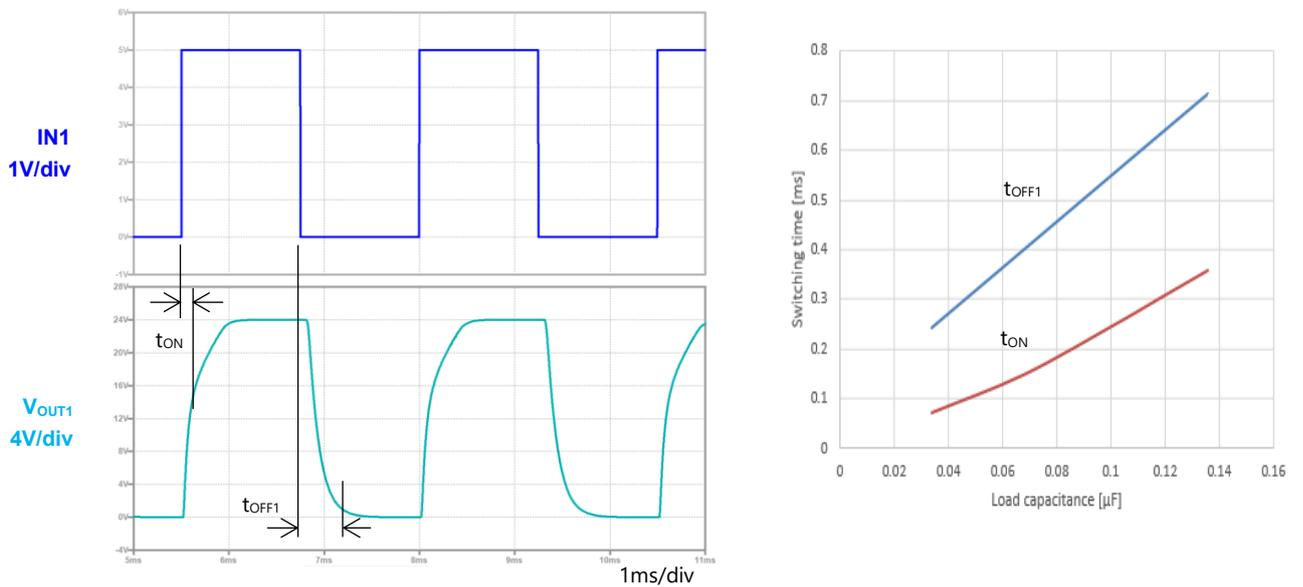
**Fig. 3.2 Switching time and load capacitance (simulation)**
