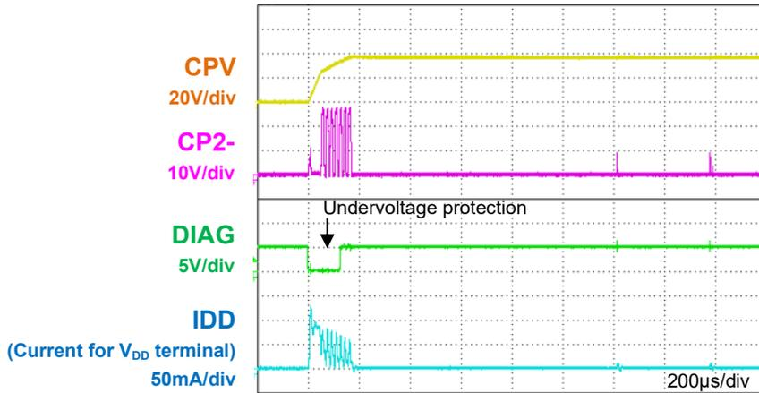
**Fig. 2.4** Rising of charge pump voltage ( $V_{CPV}$ ) after releasing standby
