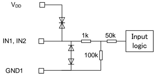
Fig. 4.2 IN1, IN2 terminal equivalent circuit
