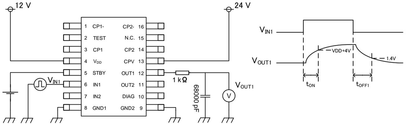
**Fig. 3.1 Switching time measurement circuit 1**
