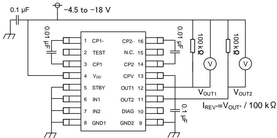
Fig. 3.4 Output current measurement circuit with power reverse connection
