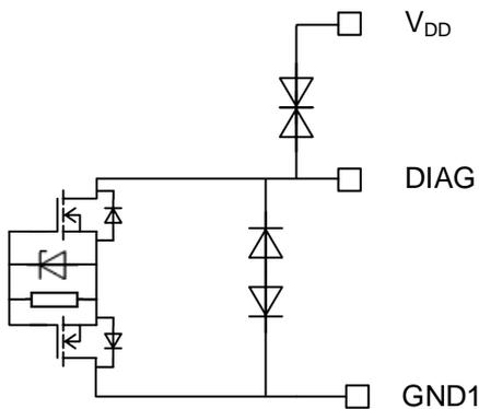
Fig. 4.7 DIAG terminal equivalent circuit
