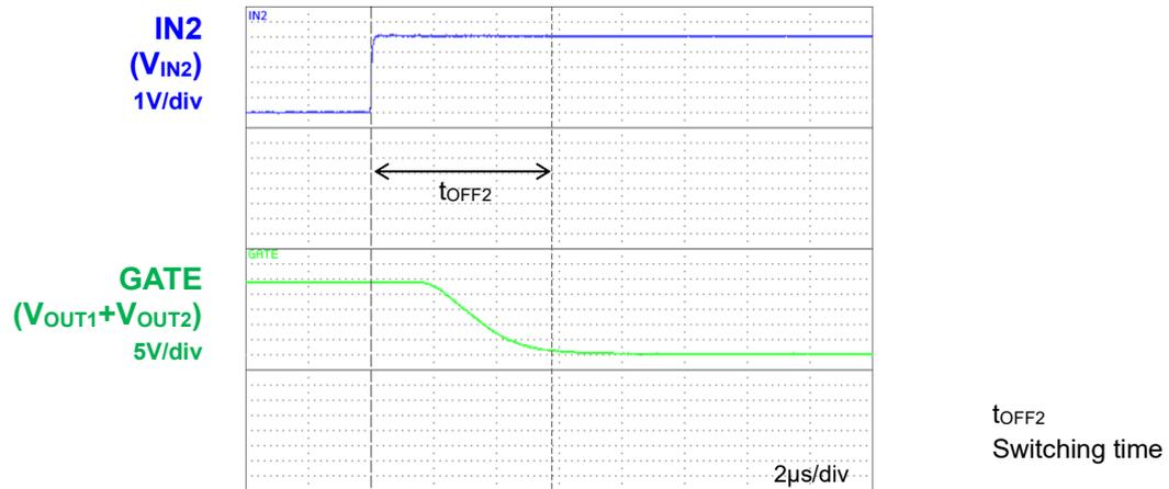
Fig. 2.3 Rapid off control waveform
