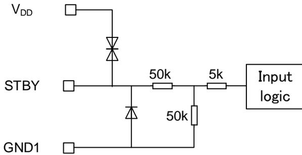
Fig. 4.1 STBY terminal equivalent circuit
