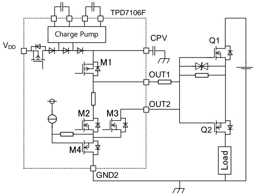
**Fig. 2.1 Control of external MOSFET**
