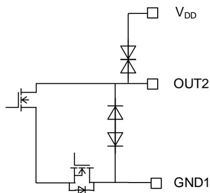
Fig. 4.6 OUT2 terminal equivalent circuit
