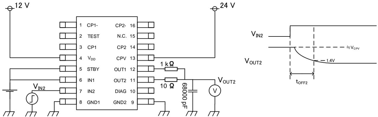
Fig. 3.3 Switching time measurement circuit 2
