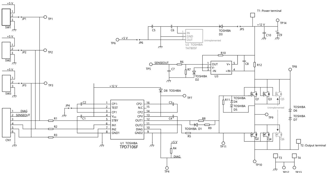
Fig. 7.4 TPD7106F evaluation board circuit diagram
