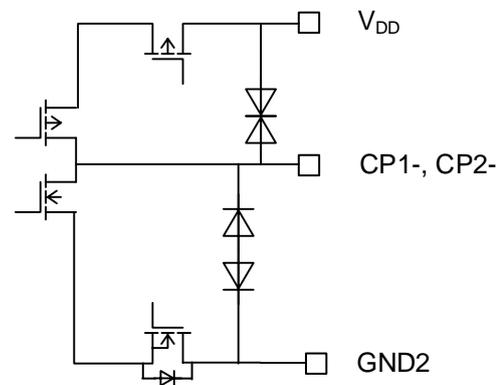
Fig. 4.4 CP1-, CP2- terminal equivalent circuit
