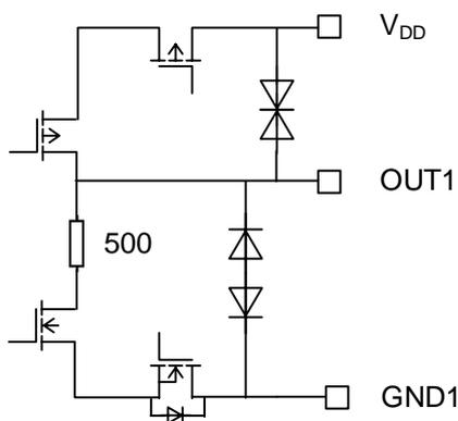
Fig. 4.5 OUT1 terminal equivalent circuit
