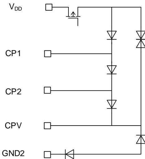
Fig. 4.3 CP1, CP2, CPV terminal equivalent circuit
