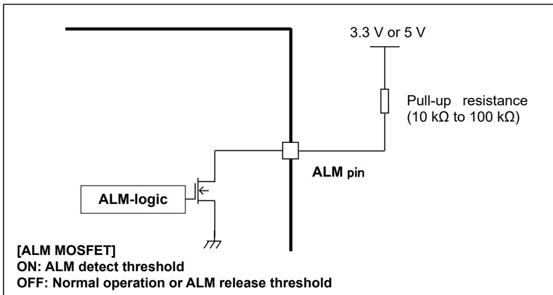
**Figure 6.5 ALM pin equivalent circuit**
