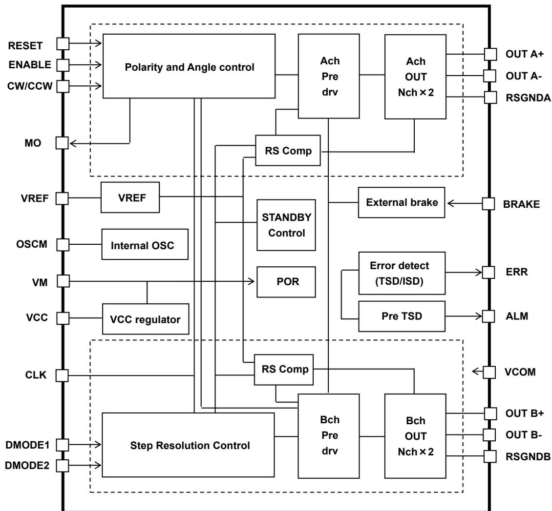
**Figure 3.1 Block Diagram**
