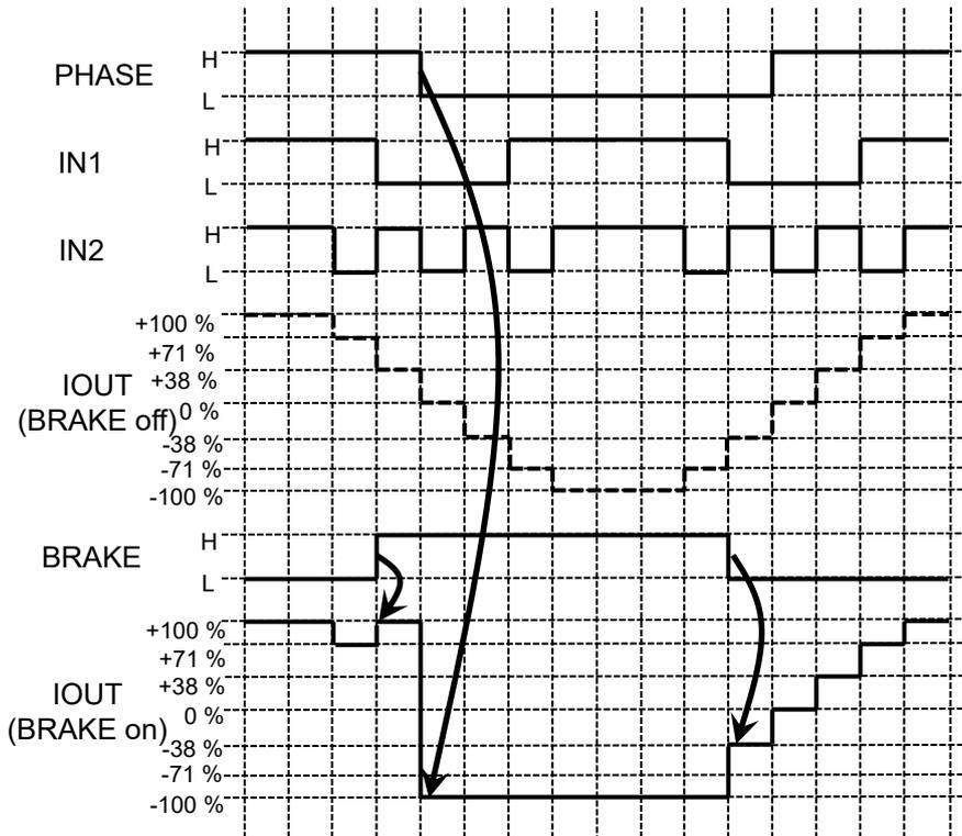
**Figure 6.5 Relation between BRAKE mode and current setting**
