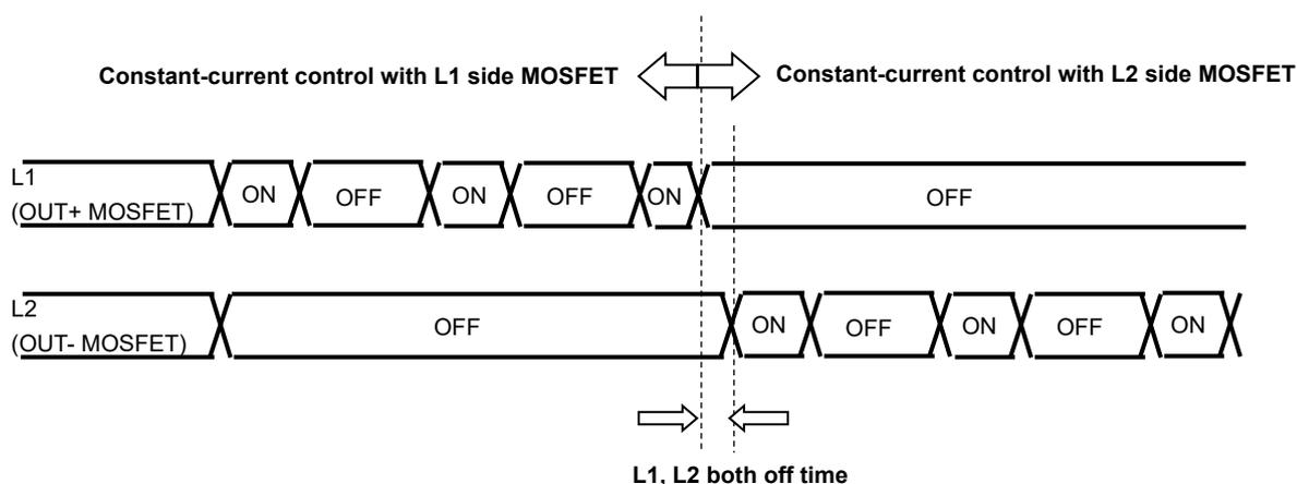
Figure 6.10 OFF TIME for PHASE switching timing chart
