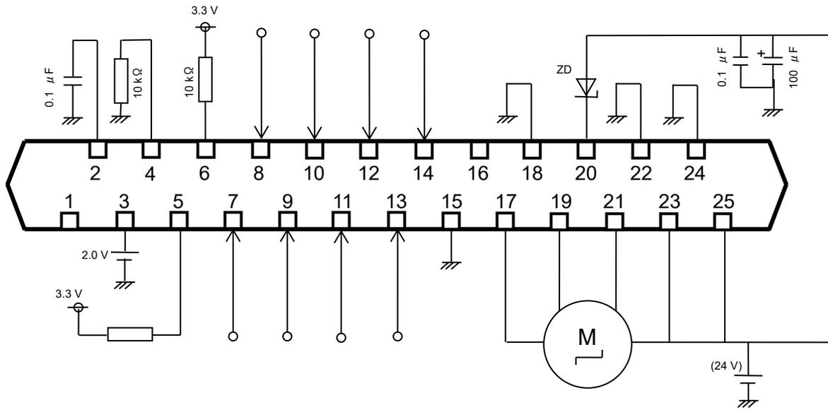
**Figure 10.1 Application Circuit Example**
