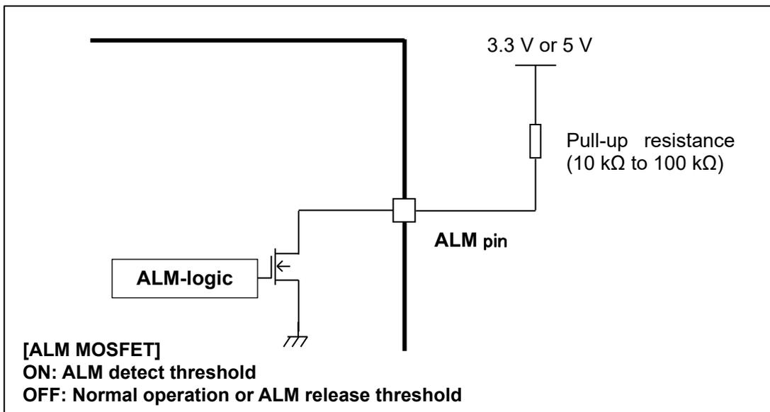
**Figure 6.8 ALM pin equivalent circuit**
