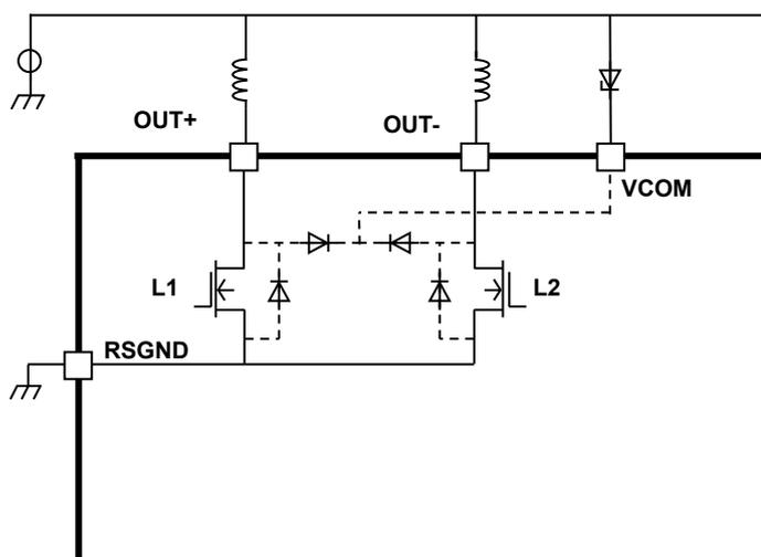
Figure 6.9 OFF TIME for PHASE switching equivalent circuit
