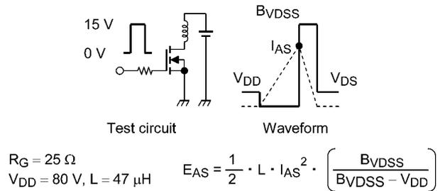
**Fig. 8.15** Test Circuit/Waveform
