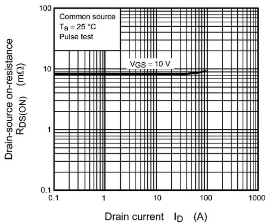
Fig. 8.5  $R_{DS(ON)} - I_D$
