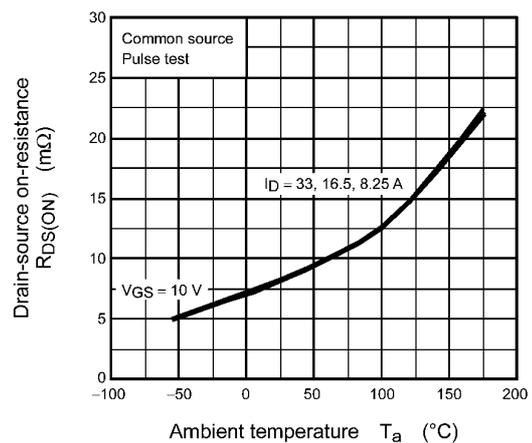
Fig. 8.6  $R_{DS(ON)} - T_a$
