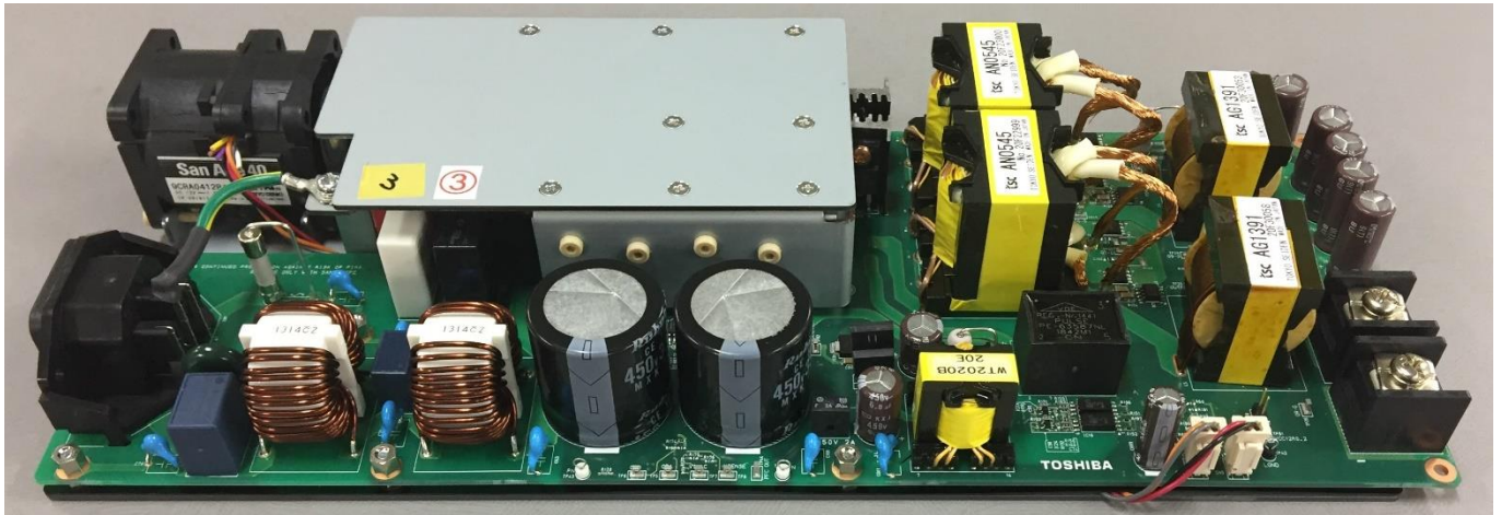
Fig. 2.1 External View of This Power supply2.21
