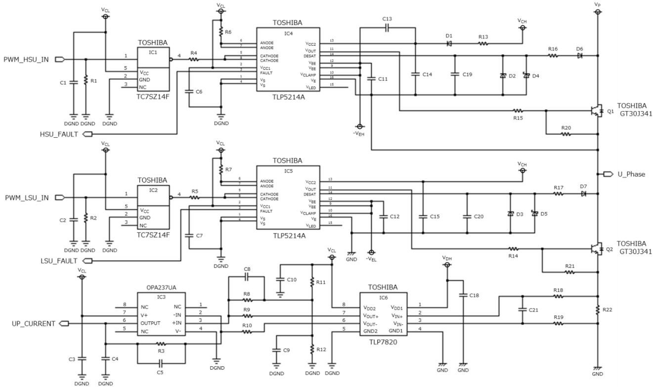
(b) U-phase diagram for inverter circuit 2
