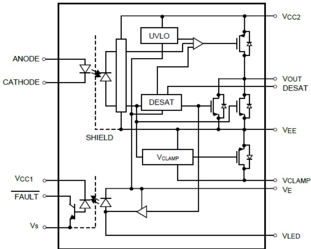
Note: 1  $\mu$ F bypass capacitor required between pins 9 ( $V_{EE}$ ) and 13 ( $V_{CC2}$ ) and between pins 13 and 16 ( $V_E$ ).
