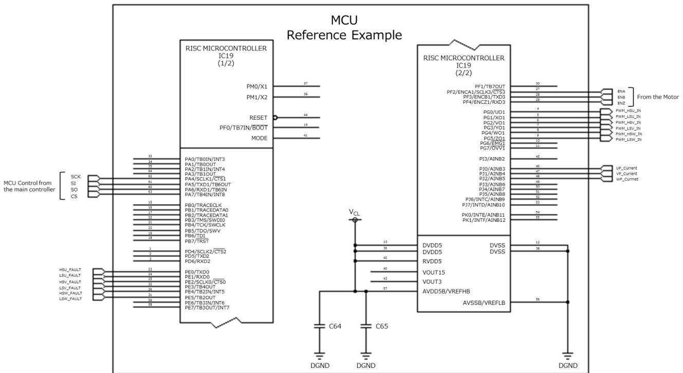
(e) MCU elements in inverter circuit 2
