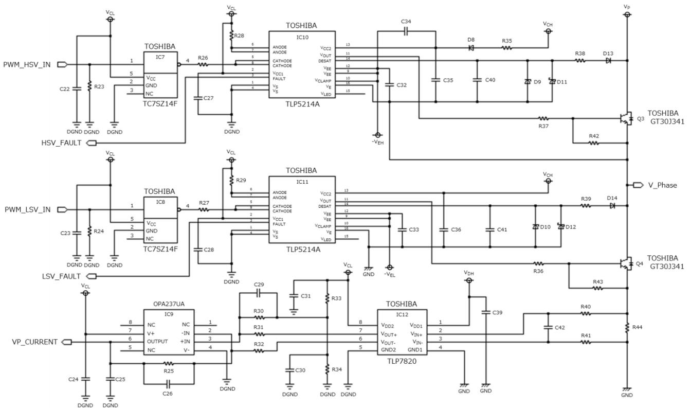
(c) V-phase diagram for inverter circuit 2
