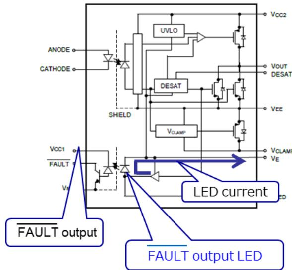
**Figure 3.7 Internal circuit diagram (operation path during fault)**
