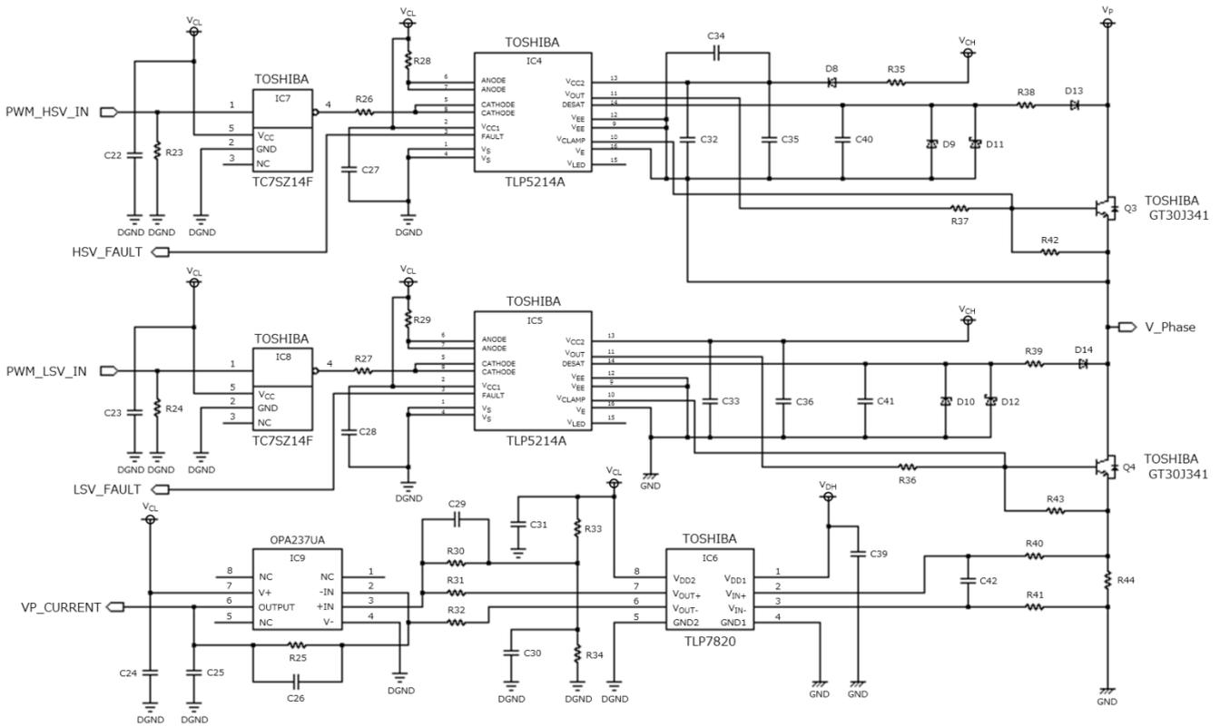
(c) V-phase diagram for inverter circuit 1
