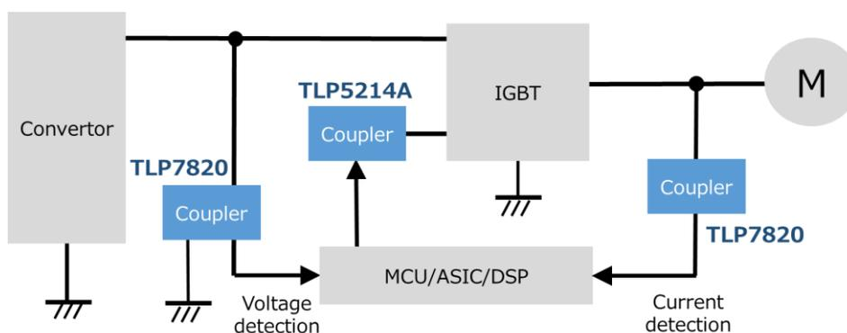
Note: Optically coupled isolation amplifier TLP7820 is used for motor phase current detection
