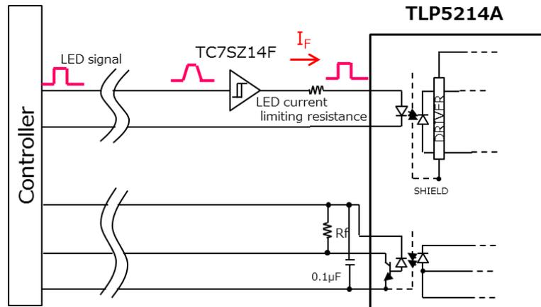
**Figure 3.4 Control signal waveform shaping**
