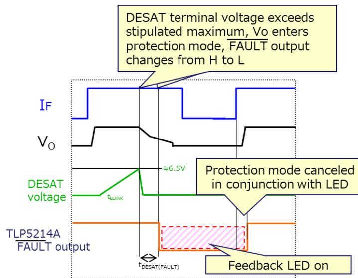
**Figure 3.8 TLP5214A timing chart (protection engaged)**
