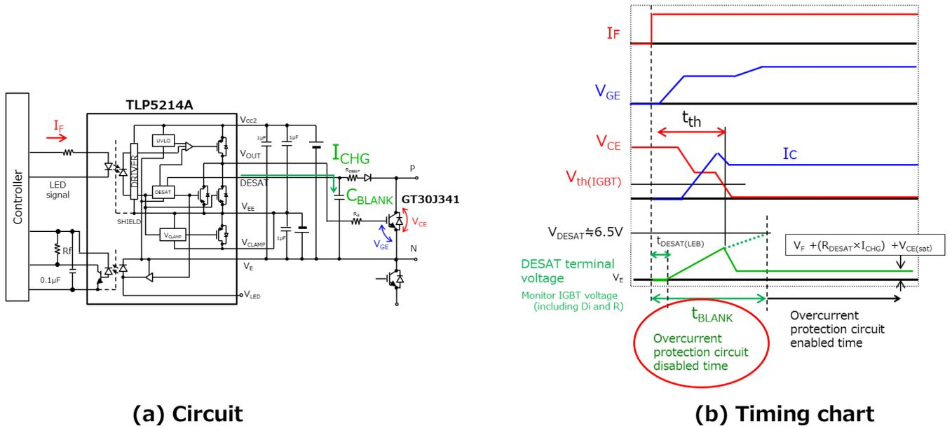
**Figure 3.1 Blanking time  $t_{BLANK}$**
