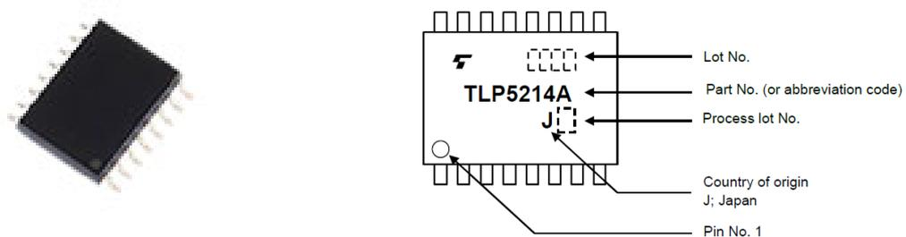
Figure 4.1 TLP5214A appearance and markings
