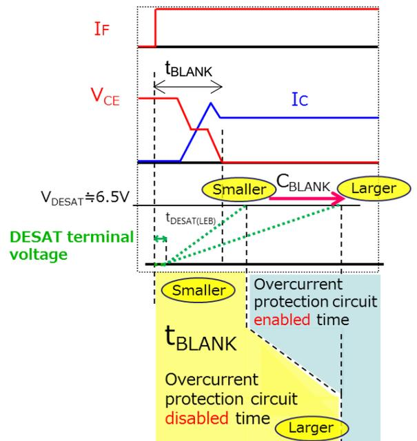
**Figure 3.2 Blanking capacity  $C_{BLANK}$  vs. blanking time  $t_{BLANK}$**
