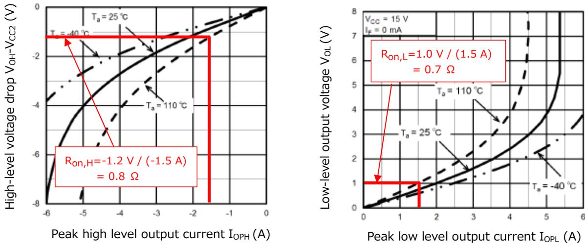
**Figure 3.6 Estimating the photocoupler output stage MOSFET on-resistance from the  $V_O$ - $I_{op}$  curve**
