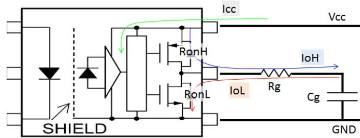
**Figure 3.5 Calculating power loss in the light receiving chip**
