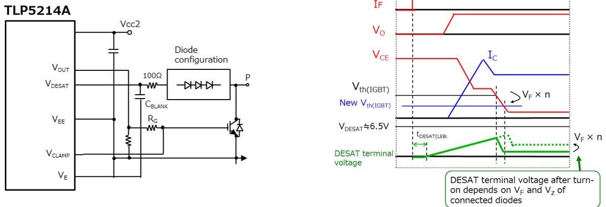
**Figure 3.3 Modifying the short-circuit threshold voltage**
