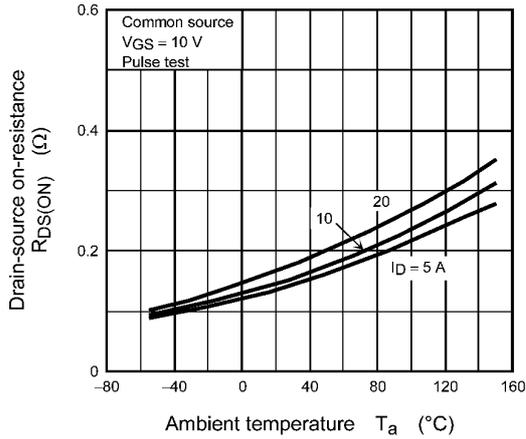
Fig. 8.7  $R_{DS(ON)} - T_a$
