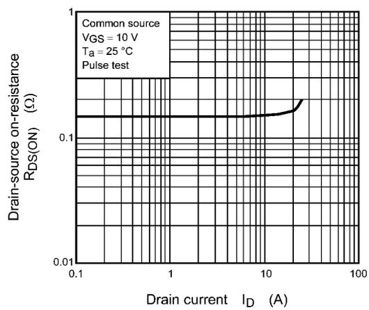
**Fig. 8.6  $R_{DS(ON)} - I_D$**
