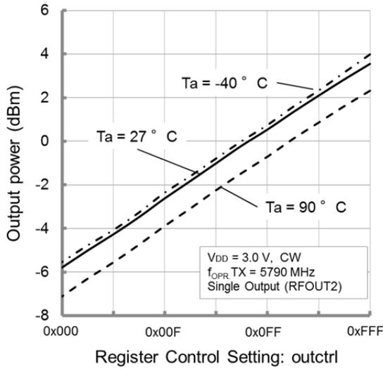
TX Output Power vs. Temperature Characteristics
