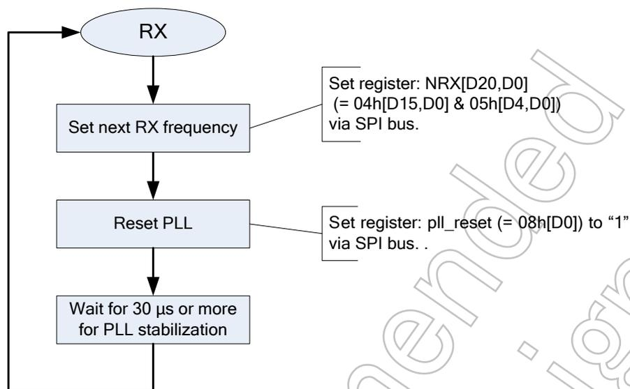
**Figure 7-15 Reception frequency change during RX state**
