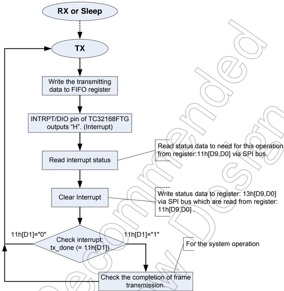
Figure 7-16 Sequence of data transmission and checking
