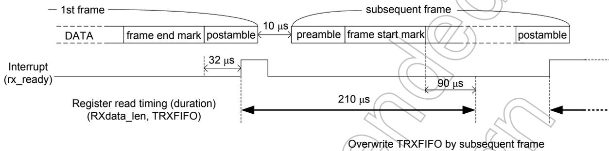
**Figure 7-20 TRXFIFO timing for two frame reception**
