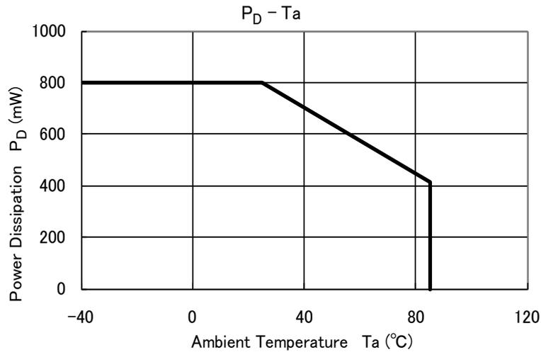
Please allow sufficient margin when designing a board pattern to fit the expected power dissipation. Also take into consideration the ambient temperature, input voltage, output current etc. and applying the appropriate derating for allowable power dissipation during operation.
