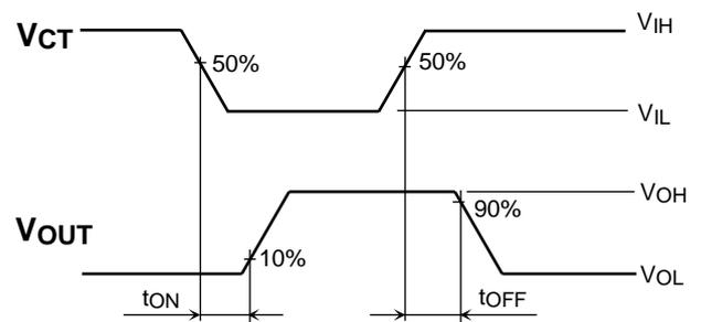
Figure 1 t<sub>r</sub>, t<sub>f</sub>, t<sub>ON</sub>, t<sub>OFF</sub> Waveforms
